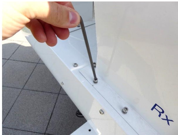
Use Allen key to fasten the air baffles.
