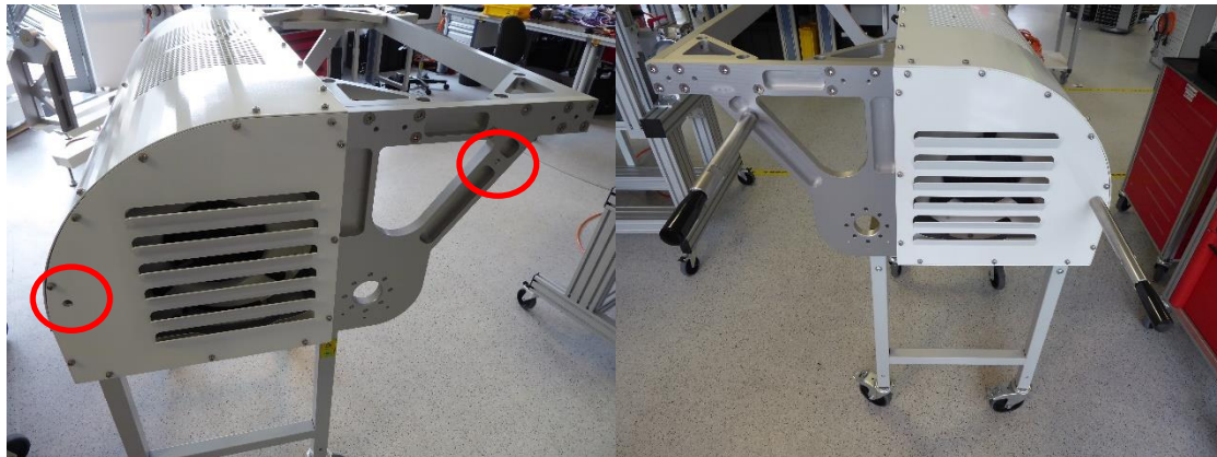
Threads for the handle mounting.
