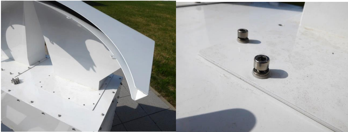
Do not tighten the screws to make the installation of the radar body easier.
