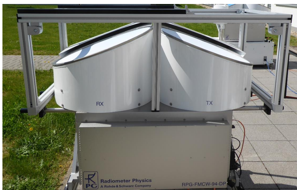
The radar with the properly mounted frame.
