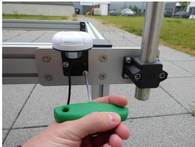
Mounting the GPS clock and the pole to the stand.
