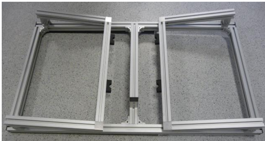
Frame for the LN2 target installation.
