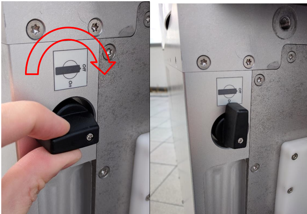
Switching on the radar.
