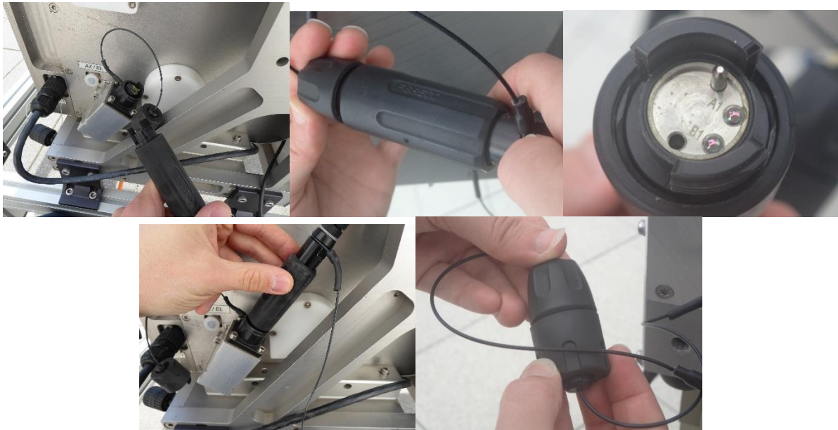
Connecting the fiber optics data cable.
