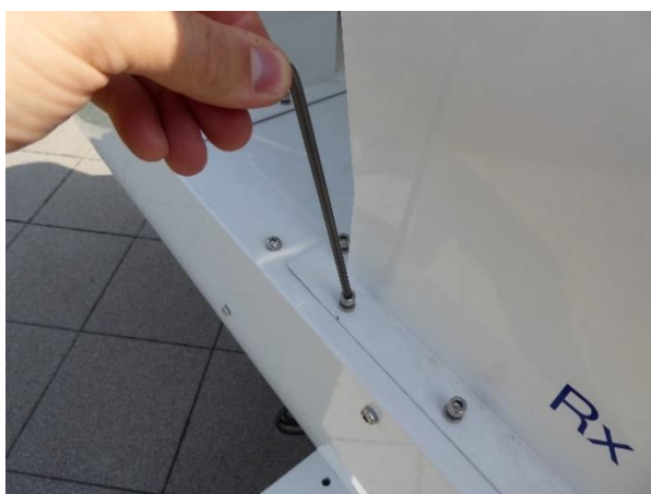
Unmounting the air baffles. Only use the Allen key!
