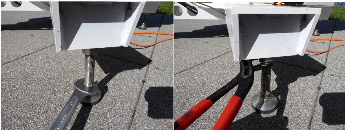
Use the elevation axis tilt reading for the horizontal alignment in both directions.
