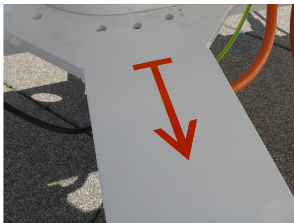
Turn the scanner in azimuth until the arrow is pointing to north direction.
