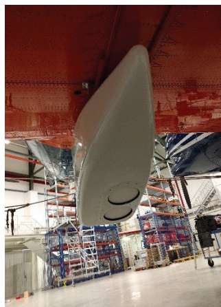
Fig. 15. Installation of the RPG radar on the Polar-5 research aircraft within the Arctic Amplification project.
