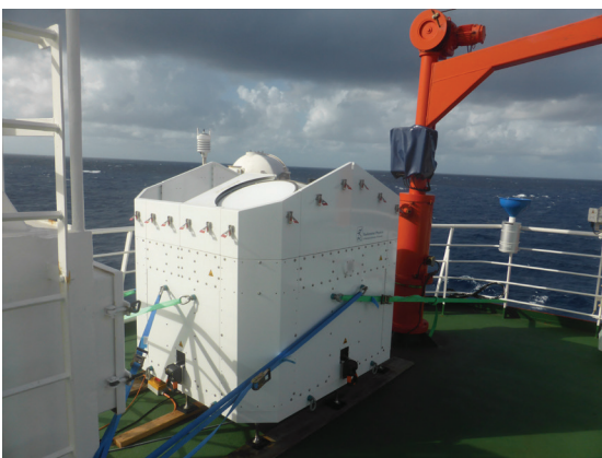
Fig. 16a. „Installation of the RPG radar with the stabilization platform and wind protection on the RV METEOR.“ Photo courtesy: University of Leipzig, Germany
