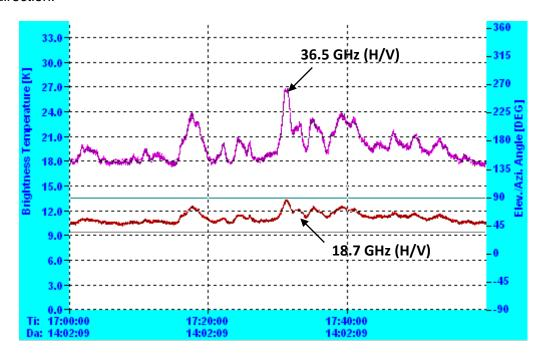
Fig. 1 Brightness Temperature time series (two frequencies, dual polarization).
