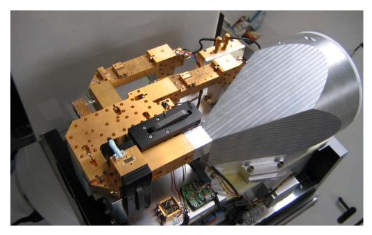
Fig. 6 RPG Double Polarization Radiometer
