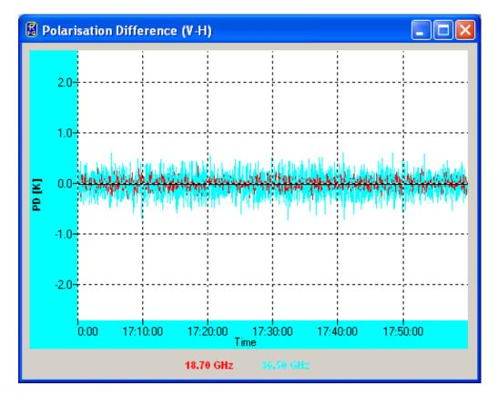
Fig. 2 Polarization difference (PD=TBv-TBh) time series for clear sky.
