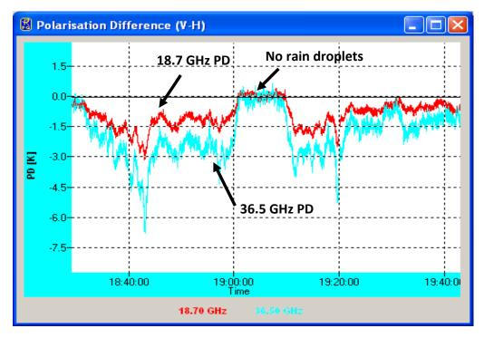
Fig. 4 Polarization Difference for rain and cloud mixtures
