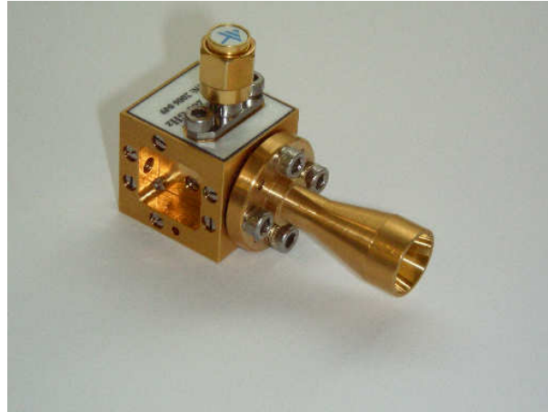
183 GHz SHM RPG-SHM-183-S1F-19 (167-200 GHz) Mixer Noise Temperature (DSB), LO: 91.5 GHz
