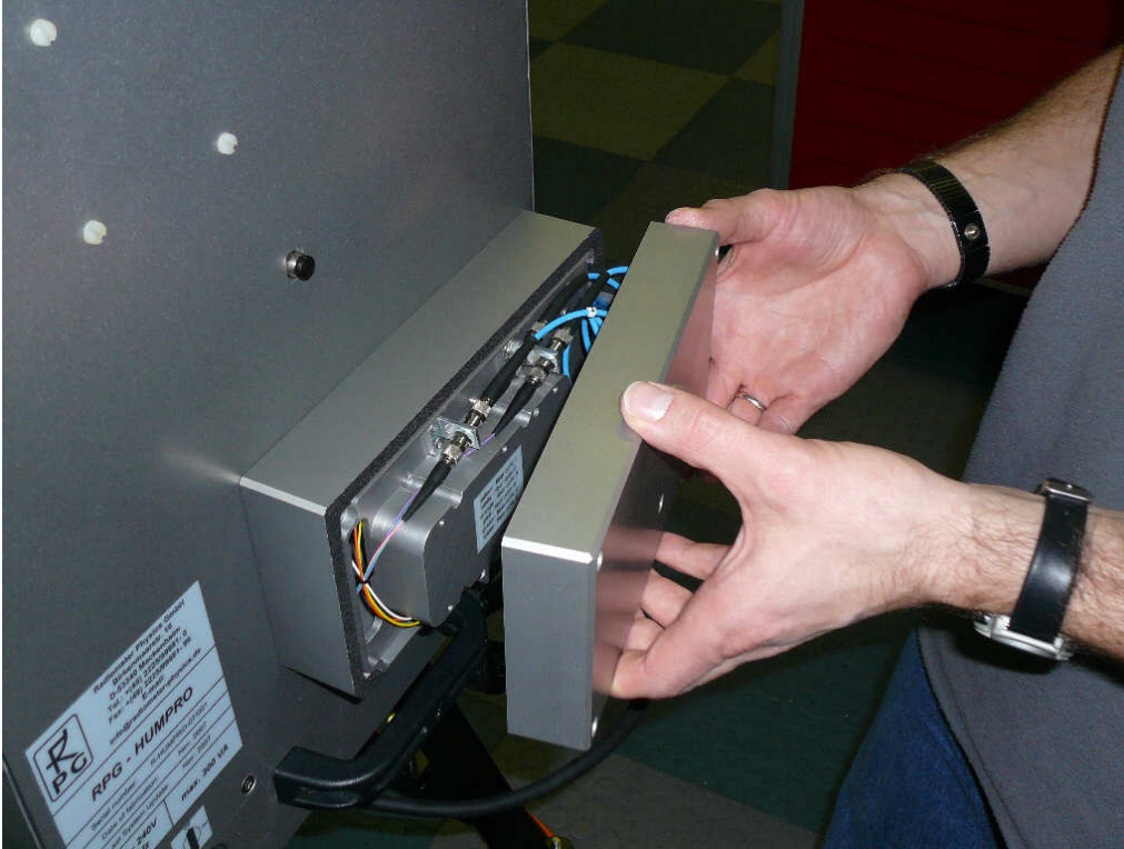
Fig.8.15a: Mounting of the lid.
