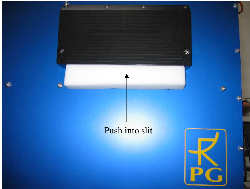
Fig.1.12: Installation of airflow reduction inlet for winter operation.
