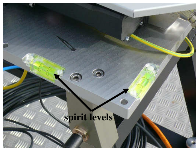
Fig.1.6b: Spirit levels on table base plate for horizontal adjustment of the stand.
