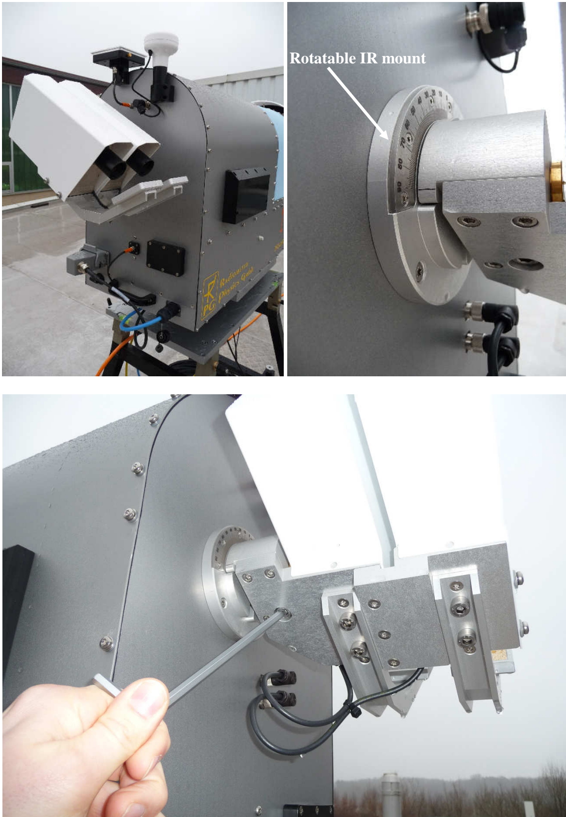
Fig.8.9: Infrared radiometer mounted to the radiometer side wall. Because of an axial mount the IR radiometer viewing angle can be changed between 0° and 90° and fixed at an arbitrary angle in this range.
