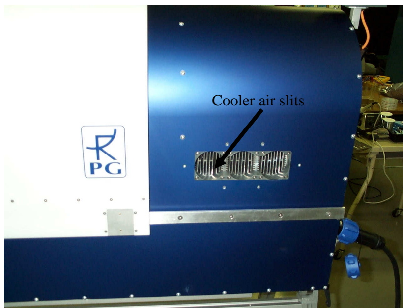
Fig.7.1: Removing the cooler cover for cleaning the cooler air inlet.
