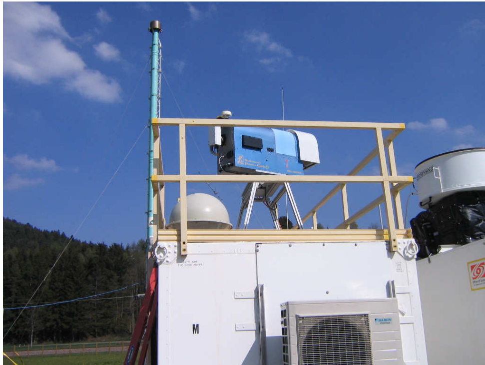
Figure 34: A HATPRO instrument with azimuth positioner during full sky scan operation at the US ARM mobile facility.
