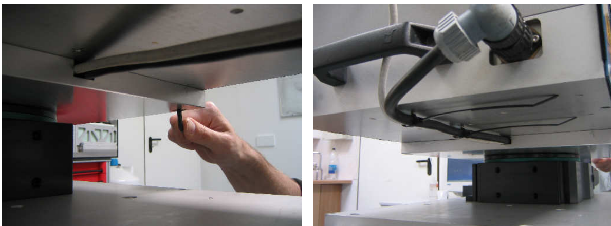
Fig.8.7: Fastening the adapter plate to the radiometer base plate and fixing the data and power cables with cable straps on the radiometer base plate.
