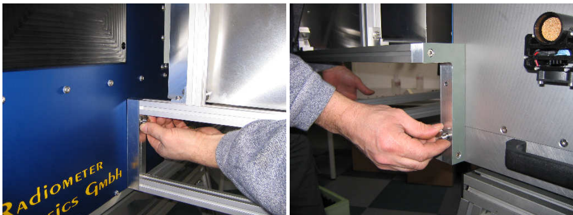
Fig.4.5a: location of mounting screws for the target frame.
