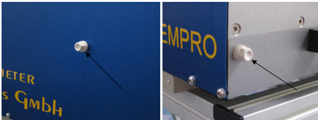
Fig.4.6: After the target frame has been unscrewed the open threads should be protected by plastic caps.
