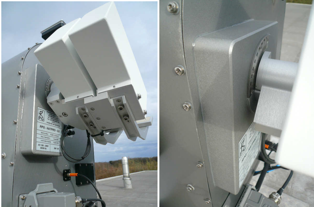
Fig.8.9b: The IRR motor drive (optional) moves the IR radiometer(s) synchronously with the internal microwave elevation mirror in the range 0° to 90°.
