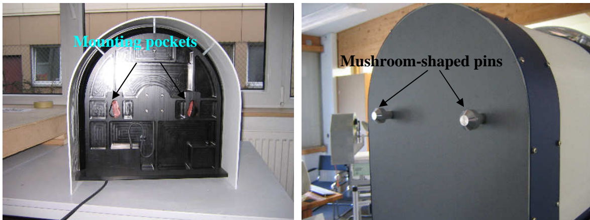
Fig.1.8: Dew blower mounting.
