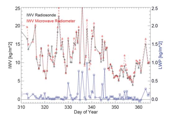
IWV measurements remain accurate even with LWP of 1000 g/m<sup>2</sup>.
