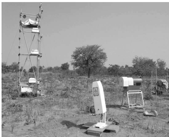
Figure 2: Setting of microwave radiometer HATPRO (right), lidar ceilometer (centre) and flux station (left) at the Nangatchori site in Benin.
