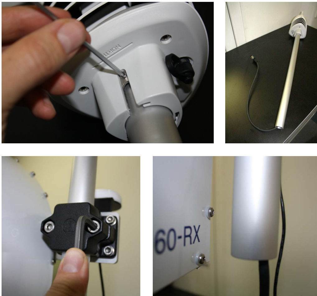
Figure 17: Mounting the weather station Vaisala WXT-520. A: Fix the station on top of the pole. The “North” arrow has to be aligned with the instrument’s side wall. B: Station, mounting pole and connecting cable. C: Use Allan key to mount the pole to the RPG-MWSC-160 receiver. D: Take care that the pole ends well above the receiver’s bottom plate level.
