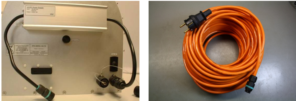
Figure 11: Left: AC power supply mounted to RPG-MWSC-160 transmitter, Right: 50 m power cable.
