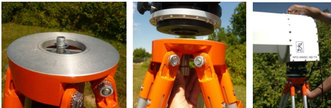
Figure 23: Fasten center bolt to mount RPG-MWSC-160 units on a tripod (single configuration).
