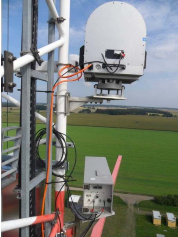
Figure 26: OMS transmitters mounted on a measurement tower in Lindenberg, Germany.
