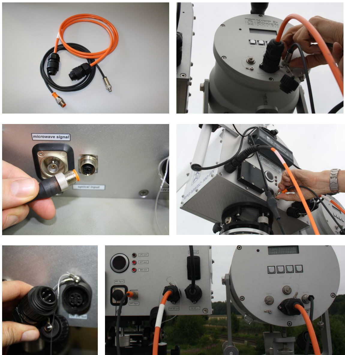
Figure 28: Example: power and data cables for the Kipp&Zonen Mk-II receiver. On the transmitter side there is only a power cable.
