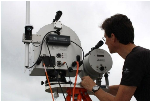
Figure 31: Example: Alignment of an OMS system.
