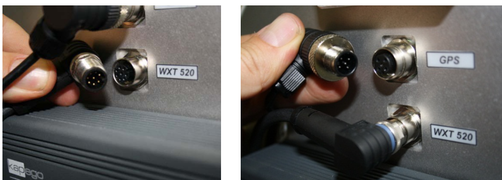
Figure 18: Connecting GPS clock and weather station.
