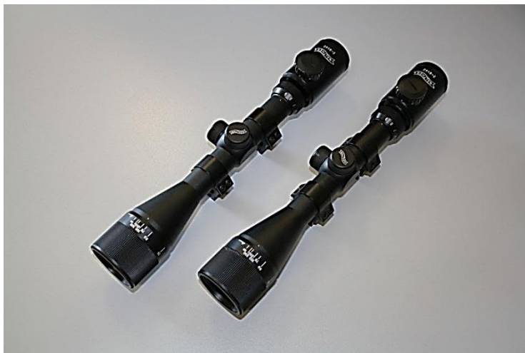
Figure 10: Alignment telescopes for the RPG-MWSC-160.
