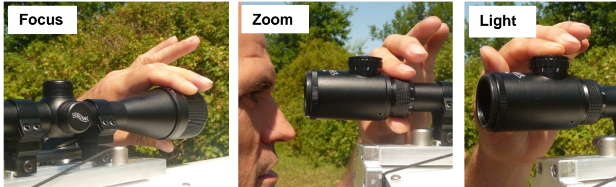
Figure 33: Adjustment of the MWS/LAS alignment telescopes.
