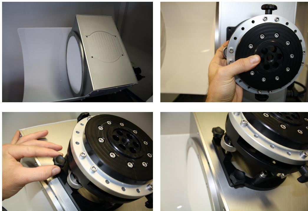
Figure 22: No tools are needed to fasten the alignment unit to the RPG-MWSC-160 units.
