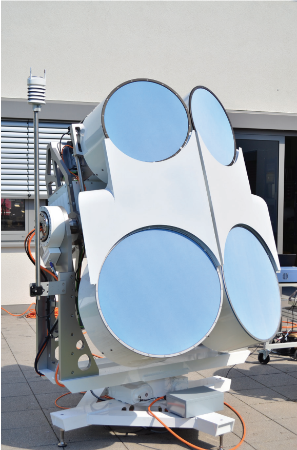
Fig. 13. Design of the dual wavelength radar system.
