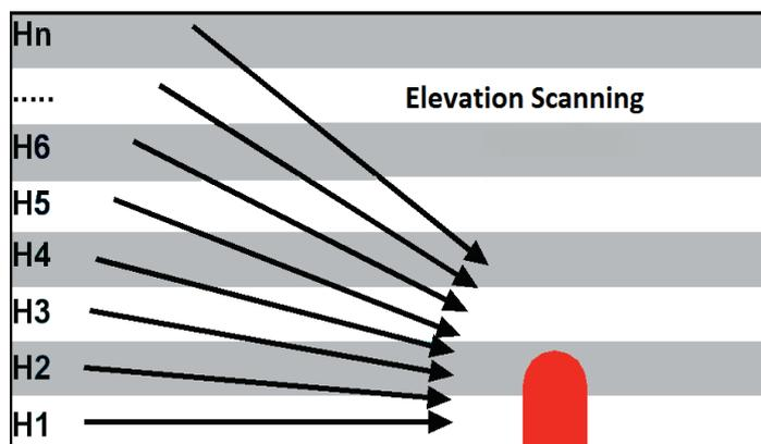
The principle of boundary layer temperature profiling is to reduce the number of contributing height levels by observing various elevation angles. The quality of boundary layer temperature profiles depends very much on the radiometer design. In order to resolve the additional height information, microwave profilers require narrow beam widths and high measurement accuracy. RPG-HATPRO radiometers comply with both criteria.
