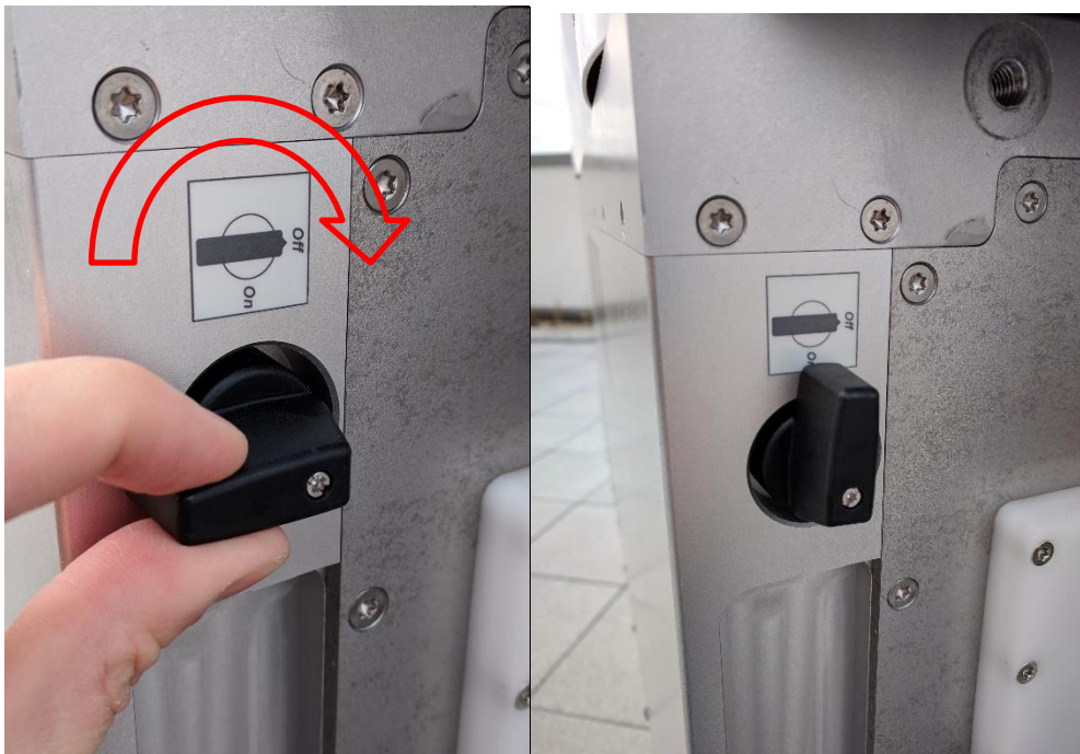
Switching on the radar.
