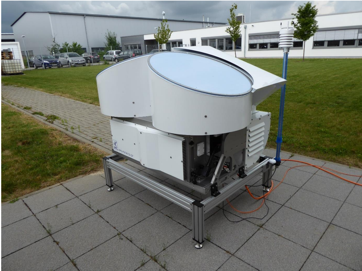
The radar body installed on the stand.
