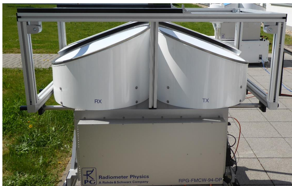
The radar with the properly mounted frame.
