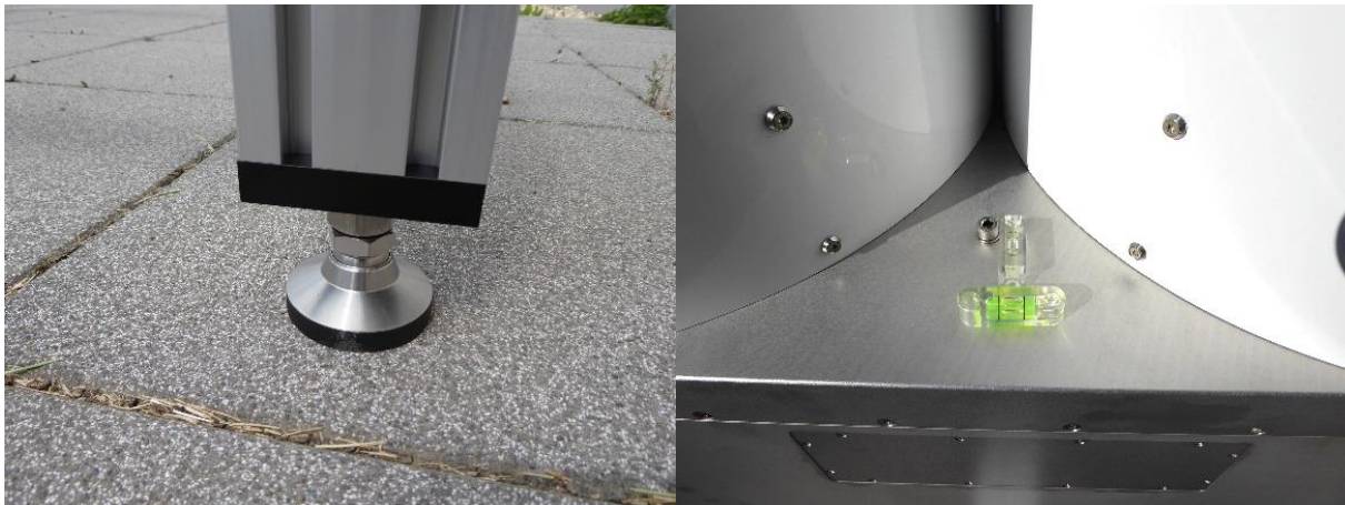
Use a small spirit level for the horizontal alignment in both directions. Place a spirit level on the reference plane between the antennas.
