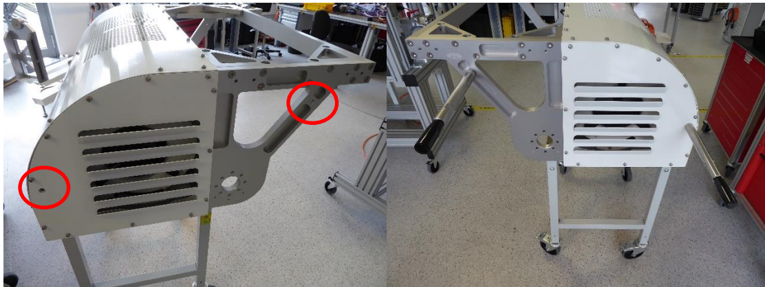
Threads for the handle mounting.
