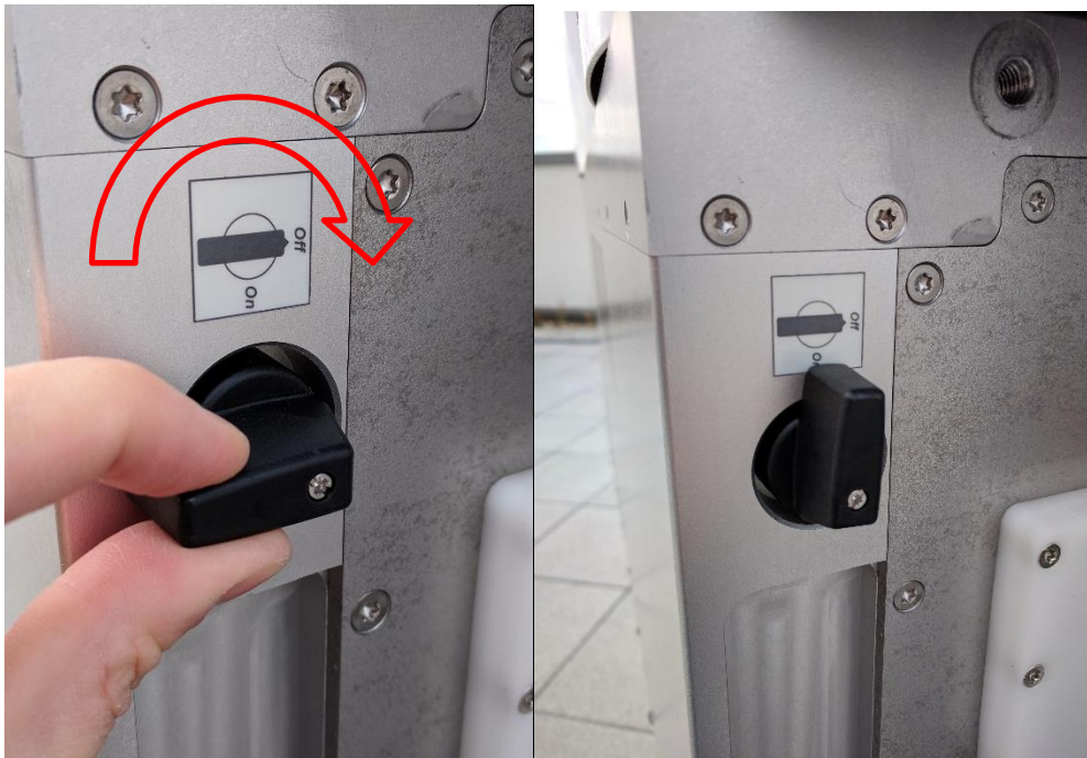
Switching on the radar.
