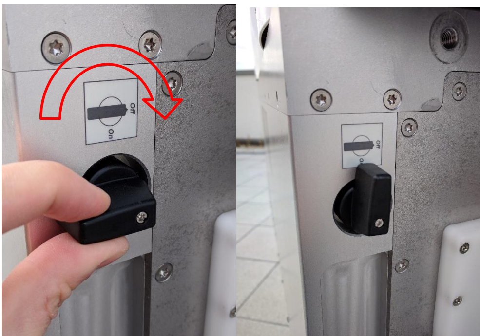
Switching on the radar.
