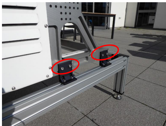
Mounting of the blower to the stand.
