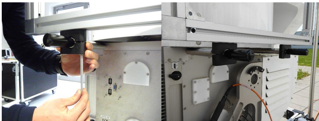
Mounting the frame to the radar housing.
