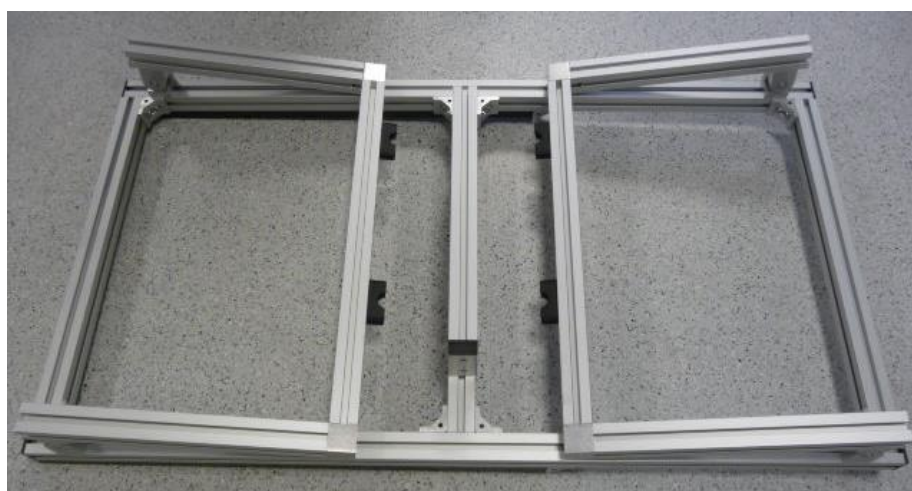
Frame for the LN2 target installation.
