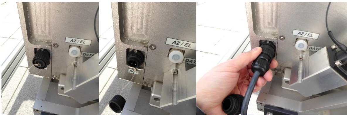
Connection of the power cable to the radar body.
