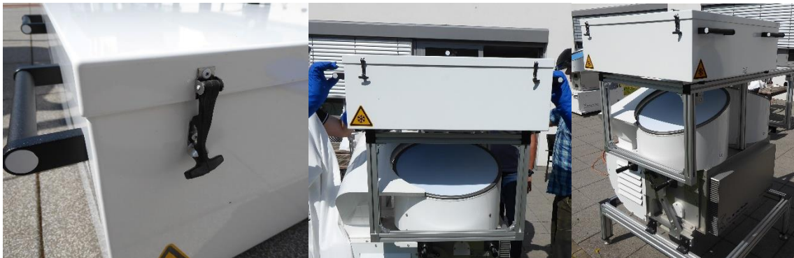
Mounting the LN2 target over the receiving antenna.
