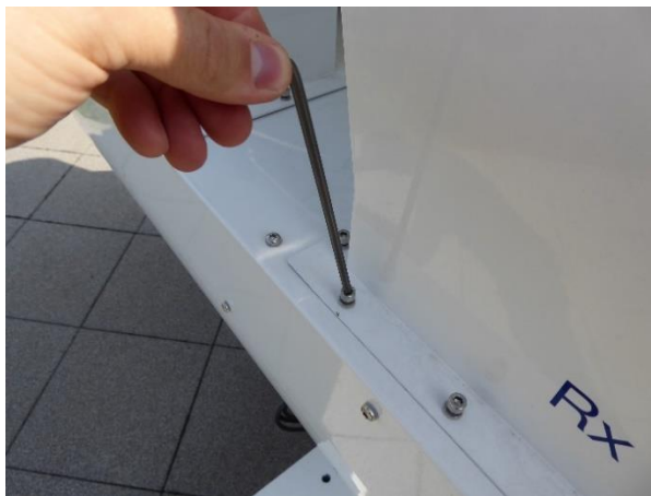
Unmounting the air guides. Only use the Allen key!
