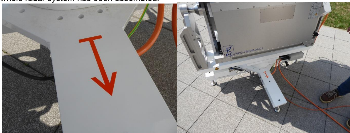
The arrow indicating 0° position of the scanner.
