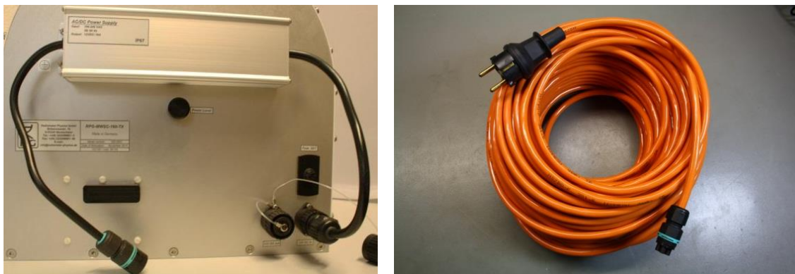
Figure 7: Left: AC power supply mounted to RPG-MWSC-160 transmitter, Right: 50 m AC power cable.
