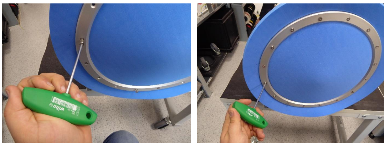
Figure 33: Compress the radome further and insert the original screws.
