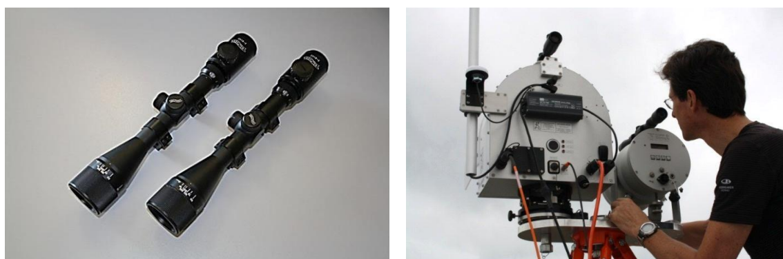
Figure 24: Example: Use the telescopes for the alignment of an OMS system.
