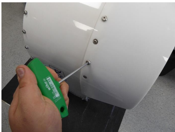
Figure 29: Dismantle rain shield.
