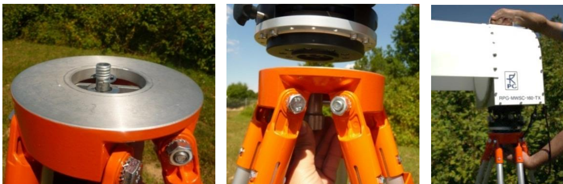
Figure 16: Fasten center bolt to mount RPG-MWSC-160 units on a tripod (single configuration).
