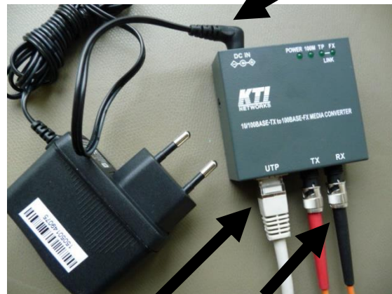
Ethernet connection Fibre-optical data cable
