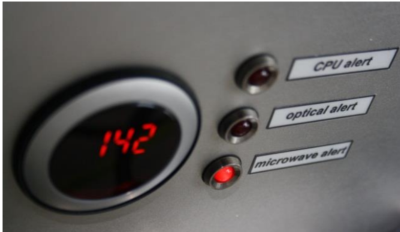
Figure 26: Receiver signal level display.
