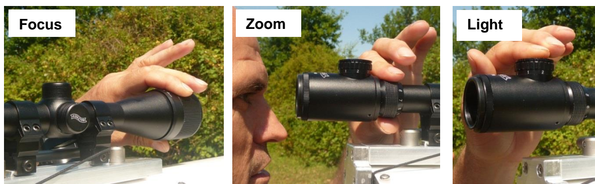
Figure 25: Adjustment of the MWS/LAS alignment telescopes.
