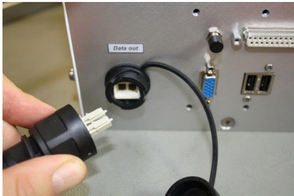
Figure 21: Setting up the fibre-optical cable for data transfer.
