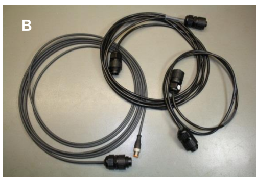
Figure 9: A: AC power cable (50 m), B: Connecting cables between MWS and LAS units for data (only receiver) and power (these cable may differ for different LAS systems), C: Data cable (50 m).
