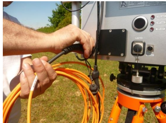
Figure 21: Setting up the fibre-optical cable for data transfer.
