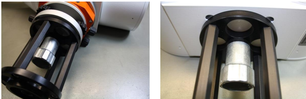
Figure 18: Mounting the height adaptors for LAS transmitter and receiver.
