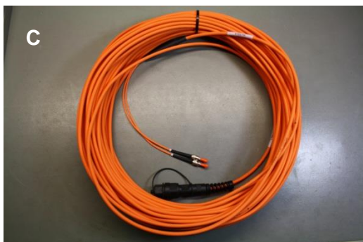
Figure 9: A: AC power cable (50 m), B: Connecting cables between MWS and LAS units for data (only receiver) and power (these cable may differ for different LAS systems), C: Data cable (50 m).
