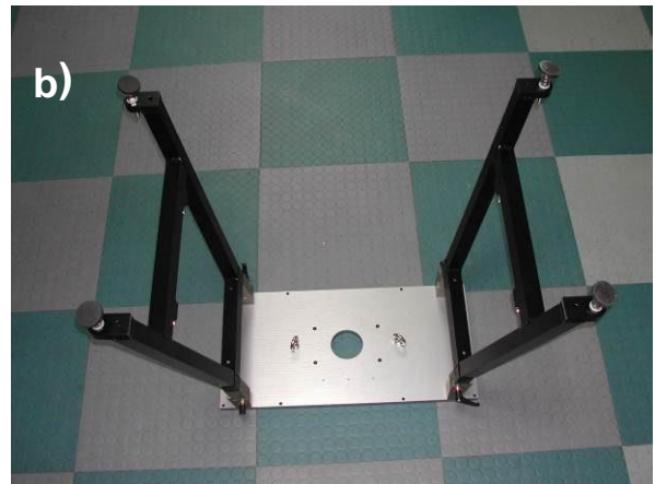
Fig.2.3.2: Open clamps and turning legs into upright position.
