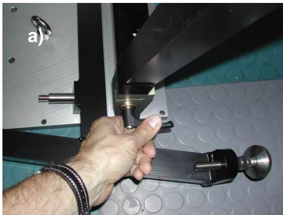
Fig.2.3.2: Open clamps and turning legs into upright position.
