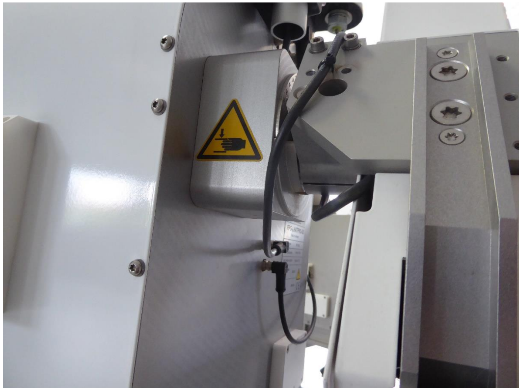
Fig.2.6.15: Motorized IRR cable wiring: 90° IR connector cable case.
