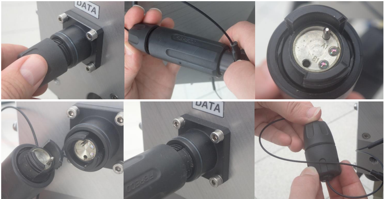
Fig.2.5.6: Connecting the fiber optics data cable.
