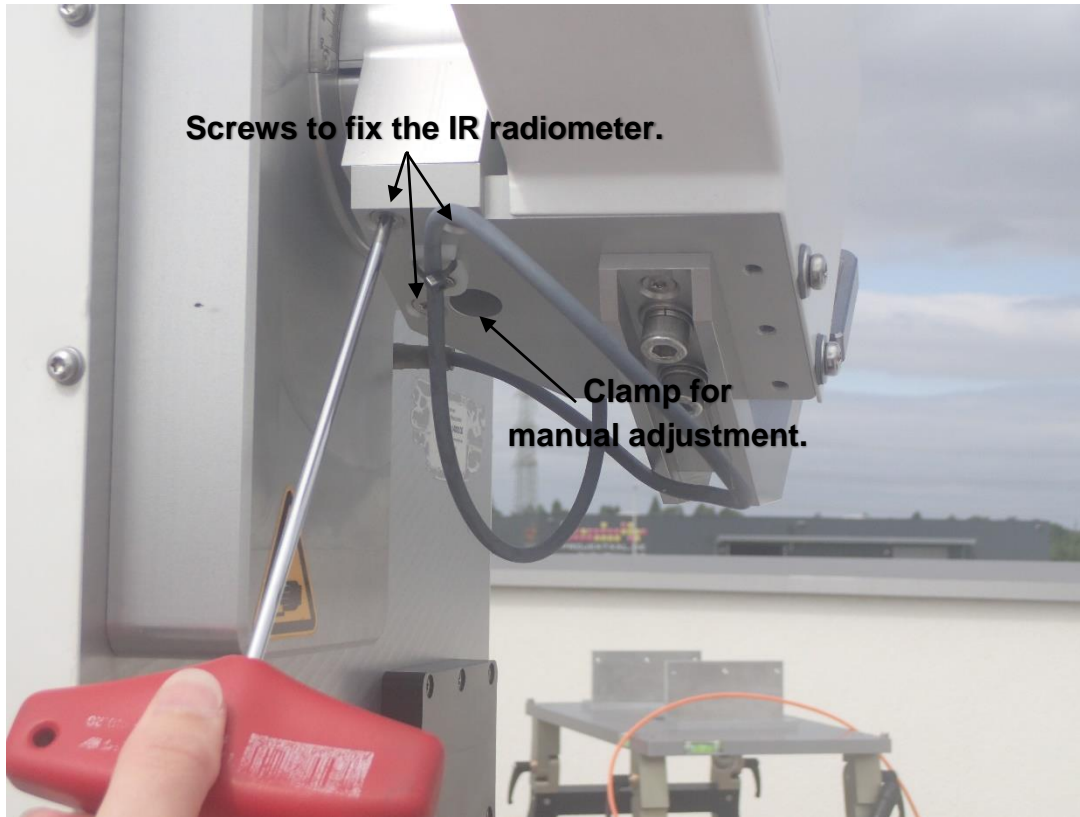
Fig. 2.6.12: Screw the IRR right with three M4 screws. The manual adjustment is then performed by loosening the clamp, rotating the IRR to the desired elevation position (use the elevation scale) and fastening the clamp again.
