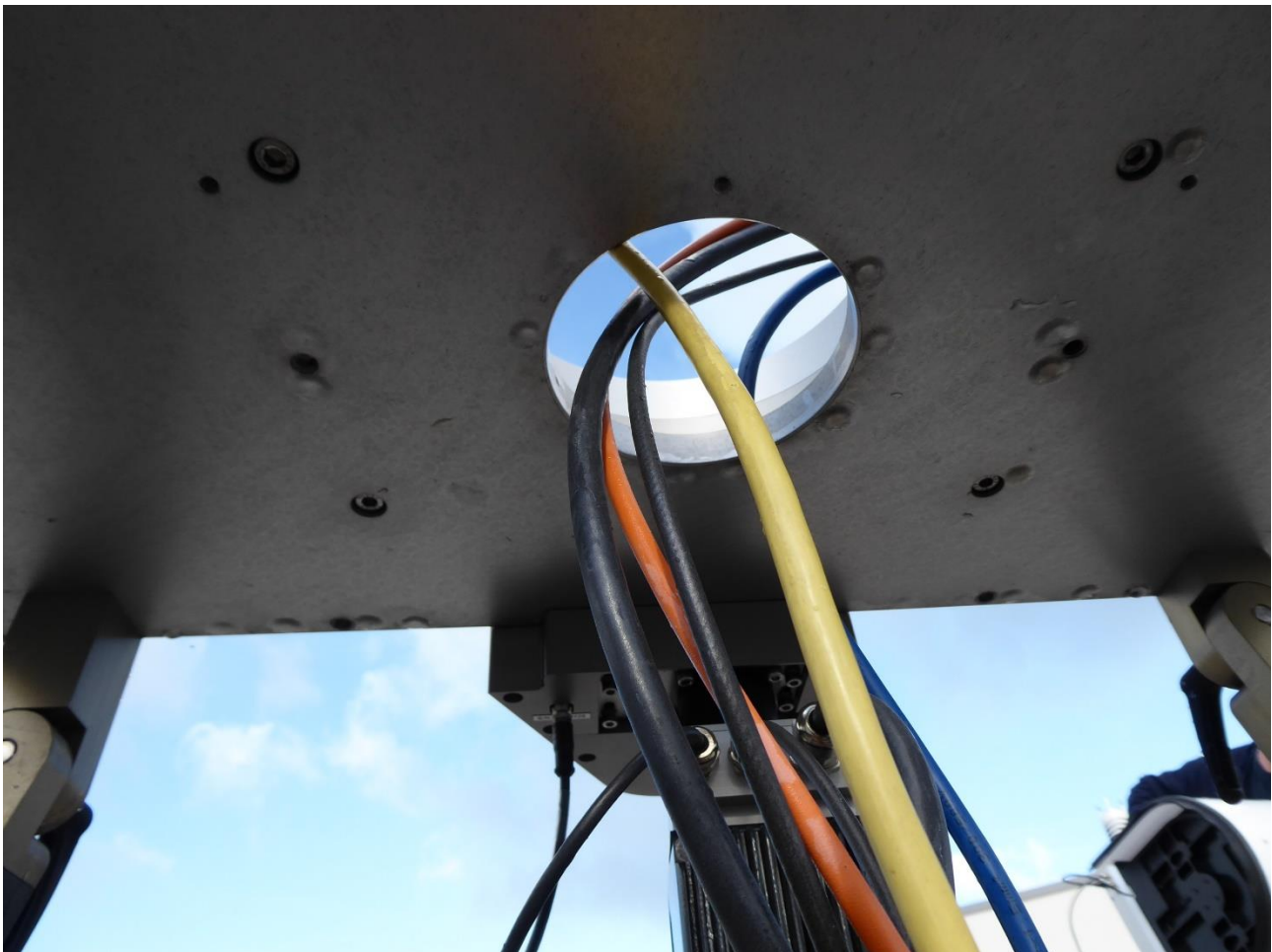
Fig. 2.4.7. Feeding the cables through center hole. Do it for AC1, AC2, DATA/AZ, fiber optic DATA, and DC/AZ.
