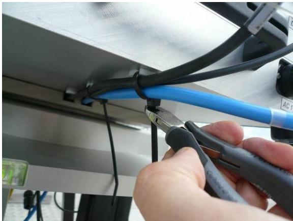
Fig.2.5.9: Fastening cables on the radiometer's bottom plate.
