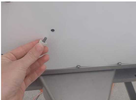
Fig4.3.7: After calibration and dismounting of the calibration target, make sure that the protection screw is inserted again.
