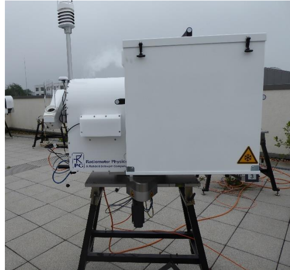
Fig. 4.3.5: Place the target on the table. Make sure that the target's sidewall marked with "R1" is facing the radiometer.
