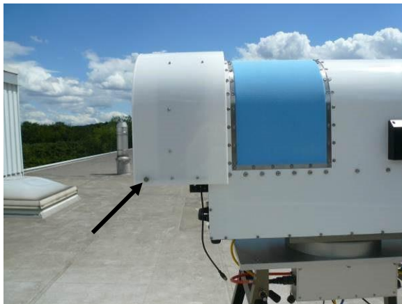
Fig.2.6.4: Remove heater mounting screws from the blower.
