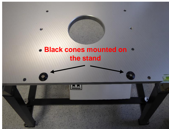
Fig.2.5.1: Black cones to be mounted only in case of no azimuth positioner
