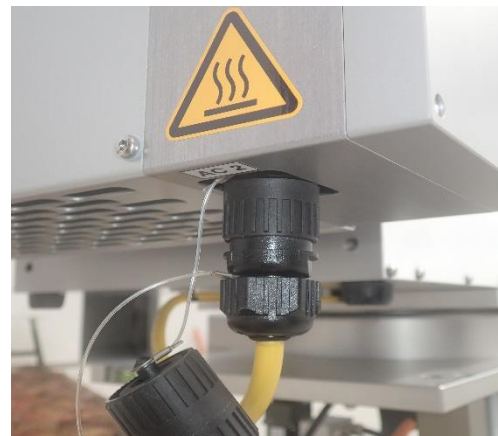
Fig.2.6.7: Connection of AC2 cable (yellow) to the heater module AC input.
