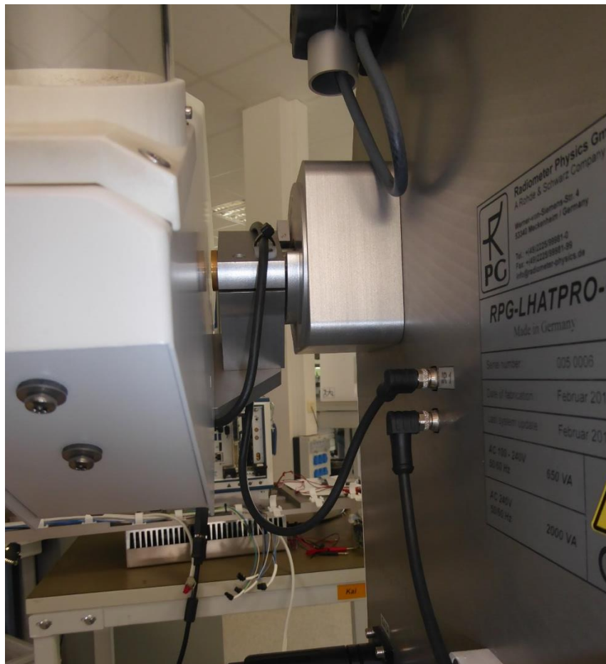
Fig.2.6.16: Motorized IRR cable wiring: 90° IR connector cable case.
