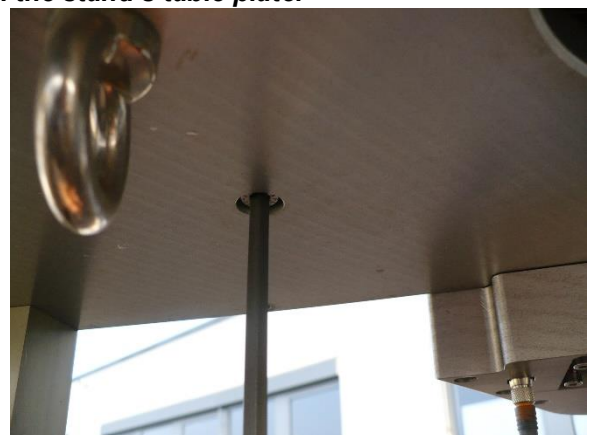
Fig.2.4.3: Fixing the azimuth drive with 6 M8x25 screws.
