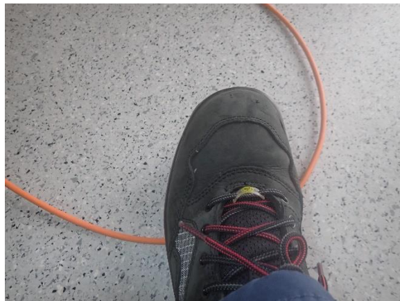
Fig.2.8.1: Avoid loops in the fiber optics cable. The curvature radius should not be less than 5 cm. Crossings of cables can lead to cable damage when stepping on it.
