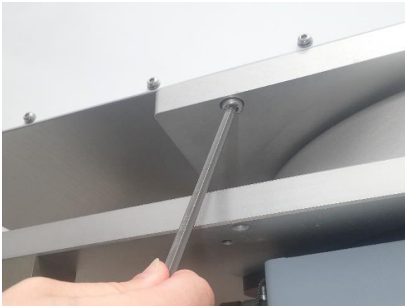
Fig.2.5.4: Use Allen key to fasten the box with four M8 screws.
