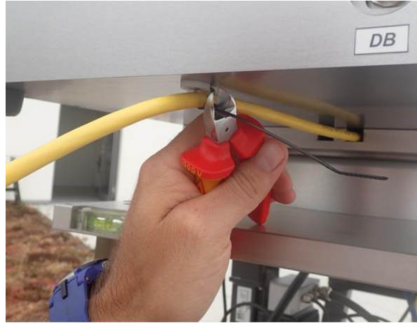
Fig.2.6.8: Fixing AC2 cable on radiometer bottom plate and cutting the cable tie.
