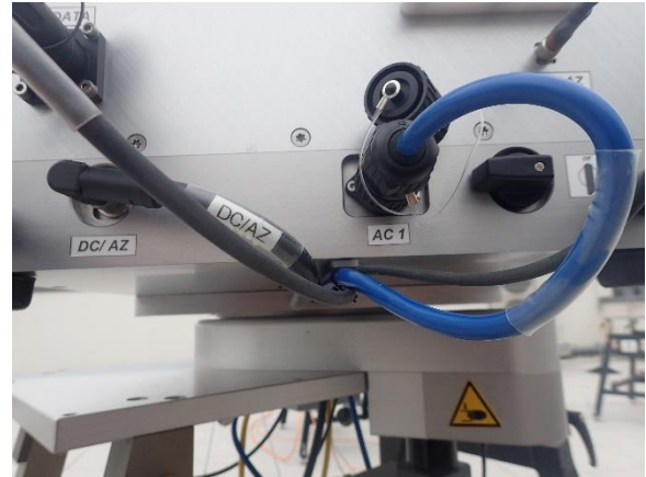
Fig.2.5.8: Pulling back the cables to adjust the cable lengths.
