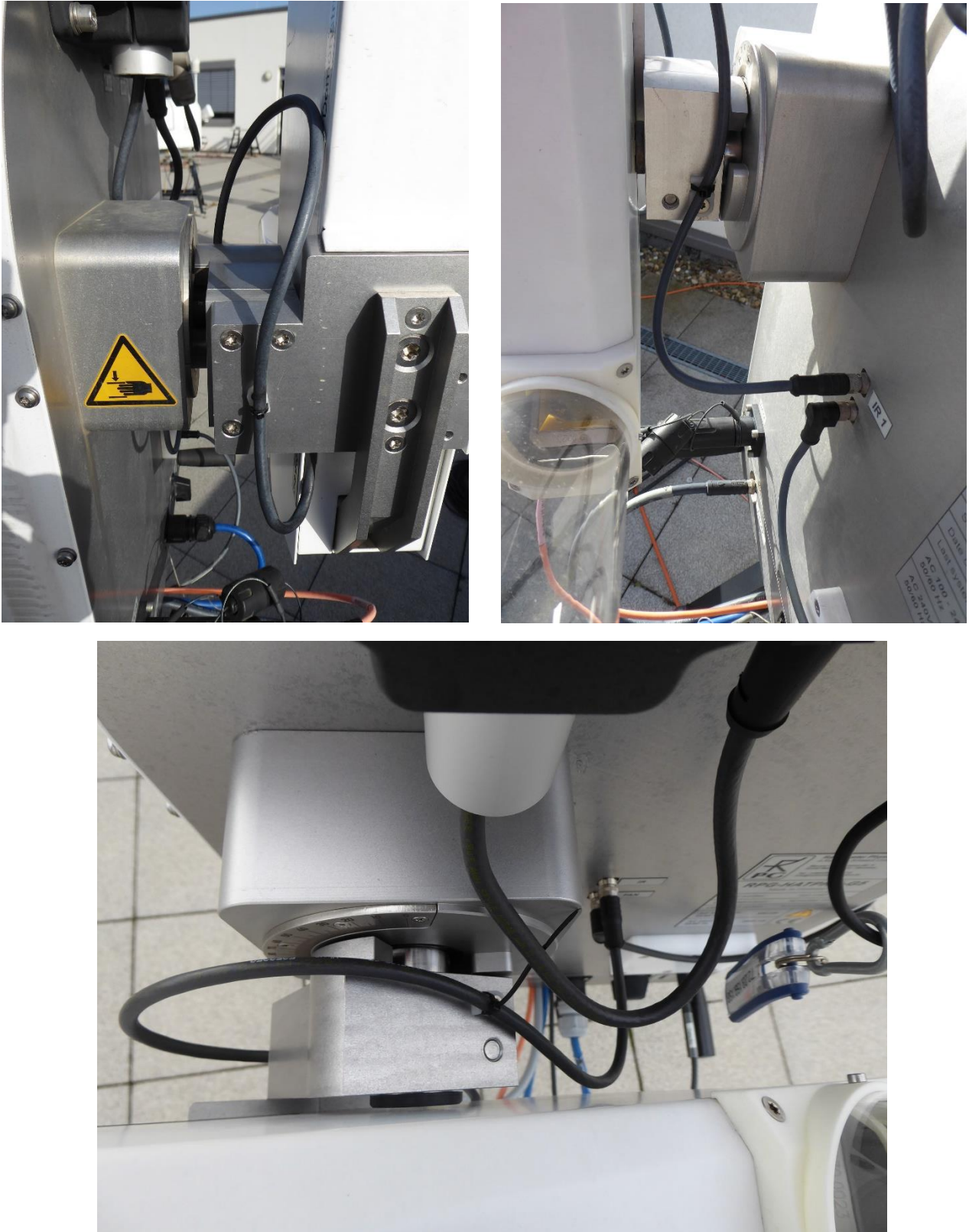
Fig.2.6.14: Motorized IRR cable wiring: straight IR connector cable case.
