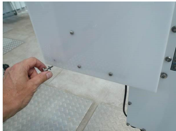
Fig.2.6.4: Remove heater mounting screws from the blower.
