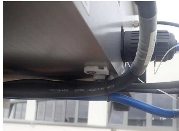
Fig.2.5.9: Fastening cables on the radiometer's bottom plate.
