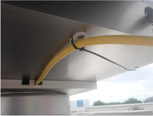
Fig.2.6.8: Fixing AC2 cable on radiometer bottom plate and cutting the cable tie.
