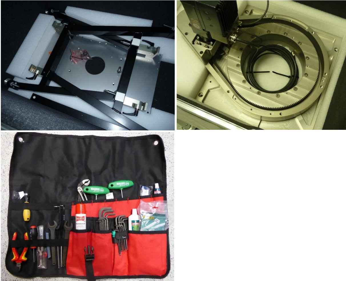
Fig.2.2.3: Folded stand and azimuth turn table both packed to their container. The toolbox includes all the tools needed to assemble, disassemble, and maintain RPG radiometers.
