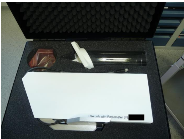
Fig.2.6.9: IR Radiometer suitcase. Fix the protective glass tube gently to the housing, using 5 torx screws M4 x 20 mm.
