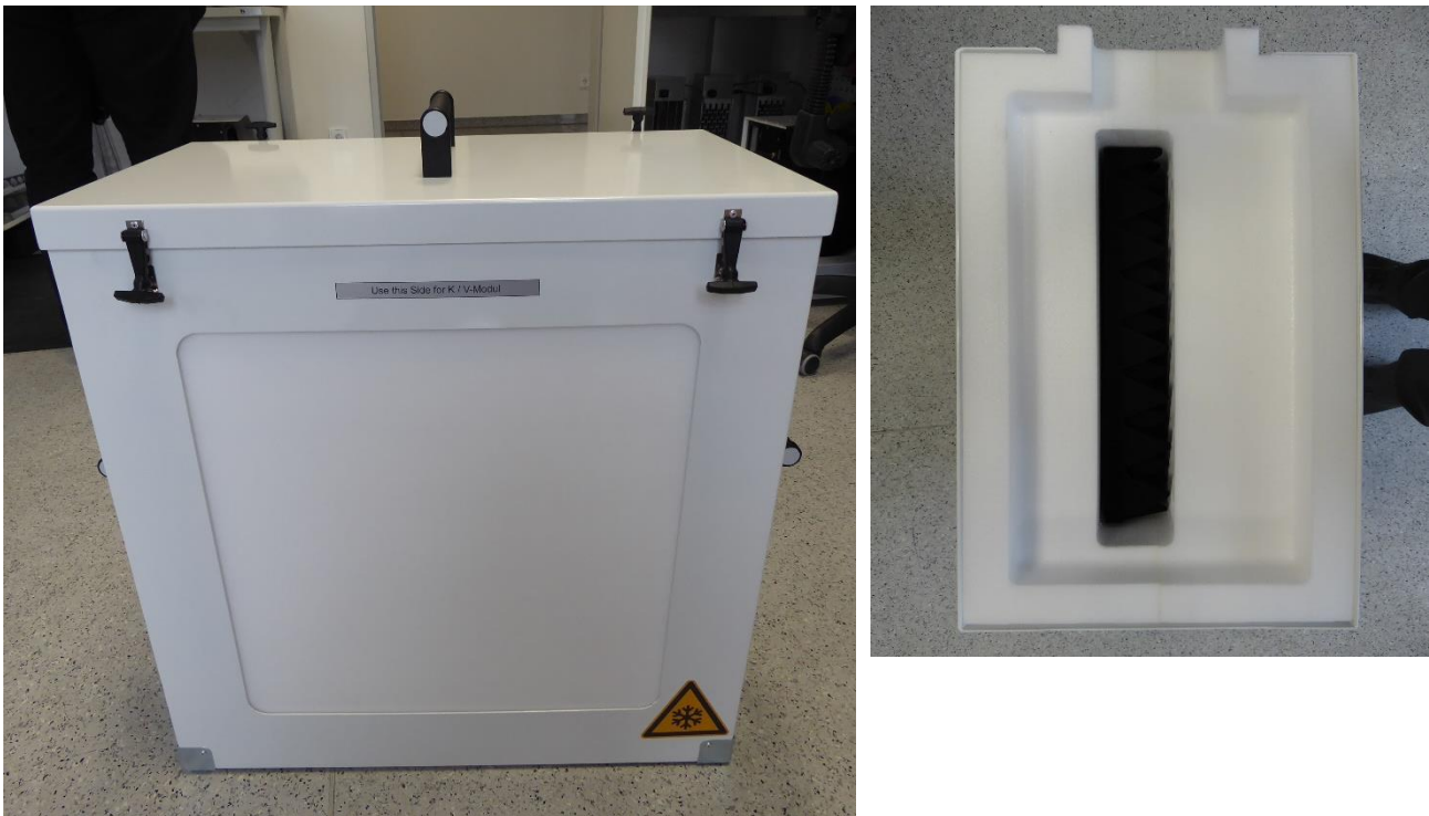
Fig. 4.3.2: Cold calibration target PT-V1 container (left) and blackbody absorber (right).
