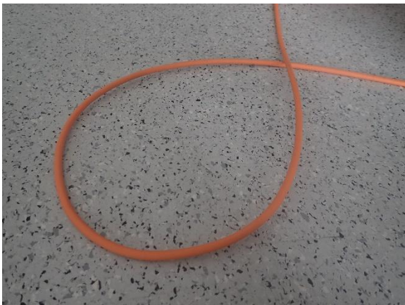
Fig.2.8.1: Avoid loops in the fiber optics cable. The curvature radius should not be less than 5 cm. Crossings of cables can lead to cable damage when stepping on it.
