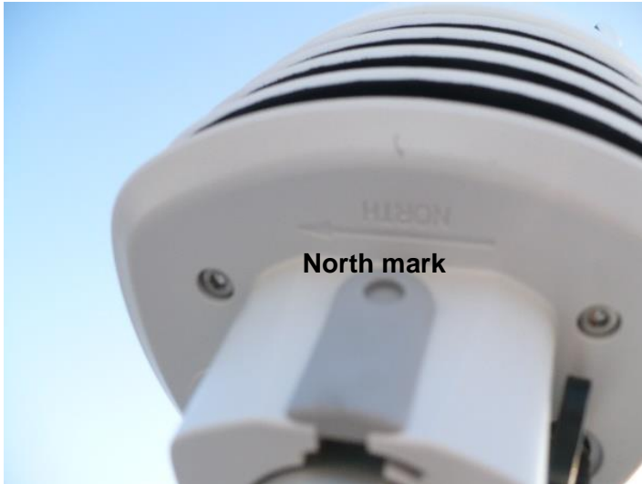
Fig.2.6.19: Orientation of north mark “N” of the Vaisala weather station.
