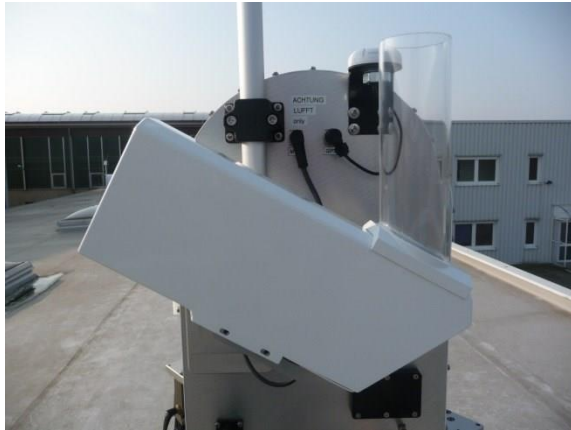
Fig.2.6.10: Infrared radiometer mounted to the radiometer side wall on manually adjustable elevation axis. Because of an axial mount the IR radiometer viewing angle can be changed between 0° and 90° and fixed at an arbitrary angle in this range.
