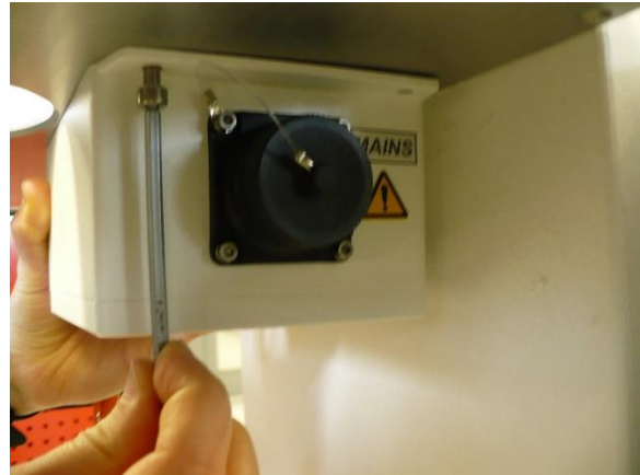
Fig. 2.4.4.: Fixing the power splitter unit to the bottom side of the stand with 4 M5x14 screws.
