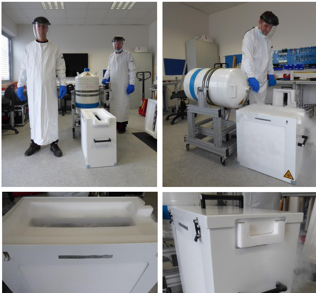
Fig. 4.3.4: Fill the calibration target with LN2 wearing suitable gloves, goggle and apron, check the filling level, close the lid, and fix the rubber fasteners.
