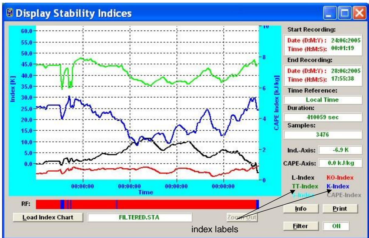
Fig.4.16: Stability index display. Information about a certain index can be obtained by double-clicking on the index label.
