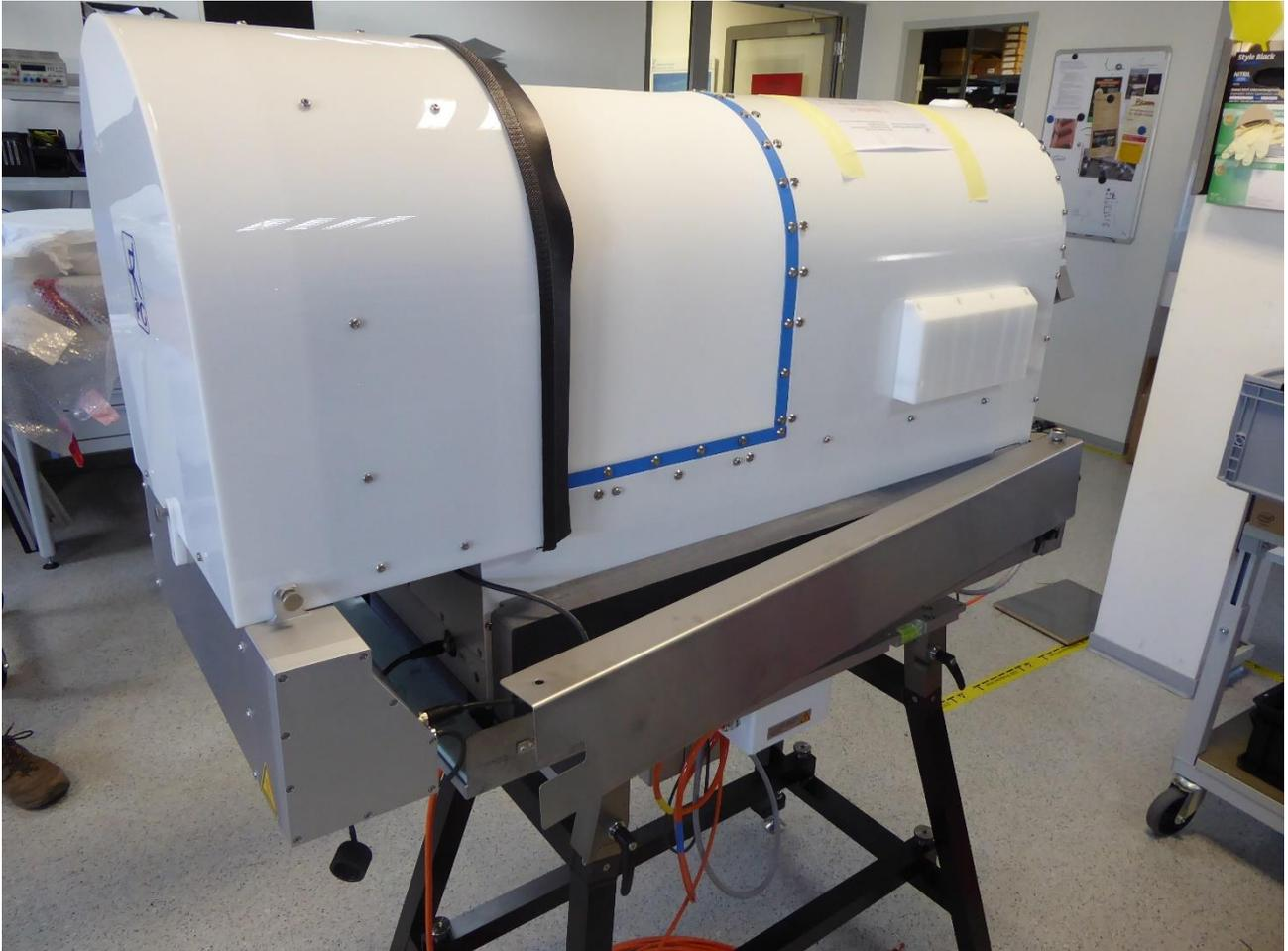
**Fig. 4.3.5: Mounting of the cold load calibration target table.**
