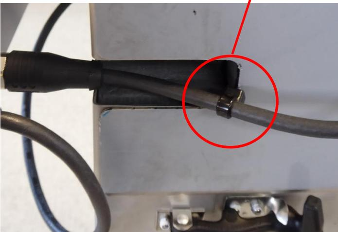
**(Fig.2.5.36): cable tie to protect the cable**
