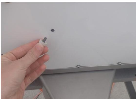
**Fig4.3.9:** After calibration and dismantling of the calibration target, make sure that the protection screw is inserted again.
