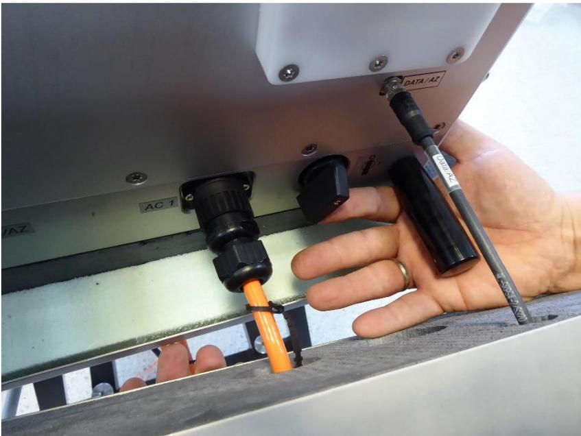
**Fig.2.5.17 fix the cables by holding the frame**
