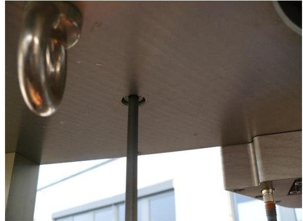
**Fig.2.4.3: Fixing the azimuth drive with 6 M8x25 screws.**
