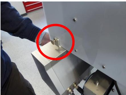
**Fig.2.5.29: heater installed to the dew blower**
