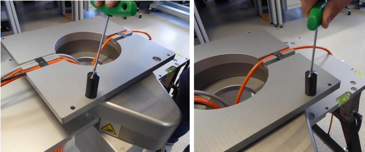
**Fig.2.4.11: mounting the long black cones to the Azimuth**
