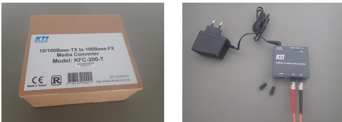
**Fig. 2.7.1: Fiber-to-LAN-TCP/IP converter.**
