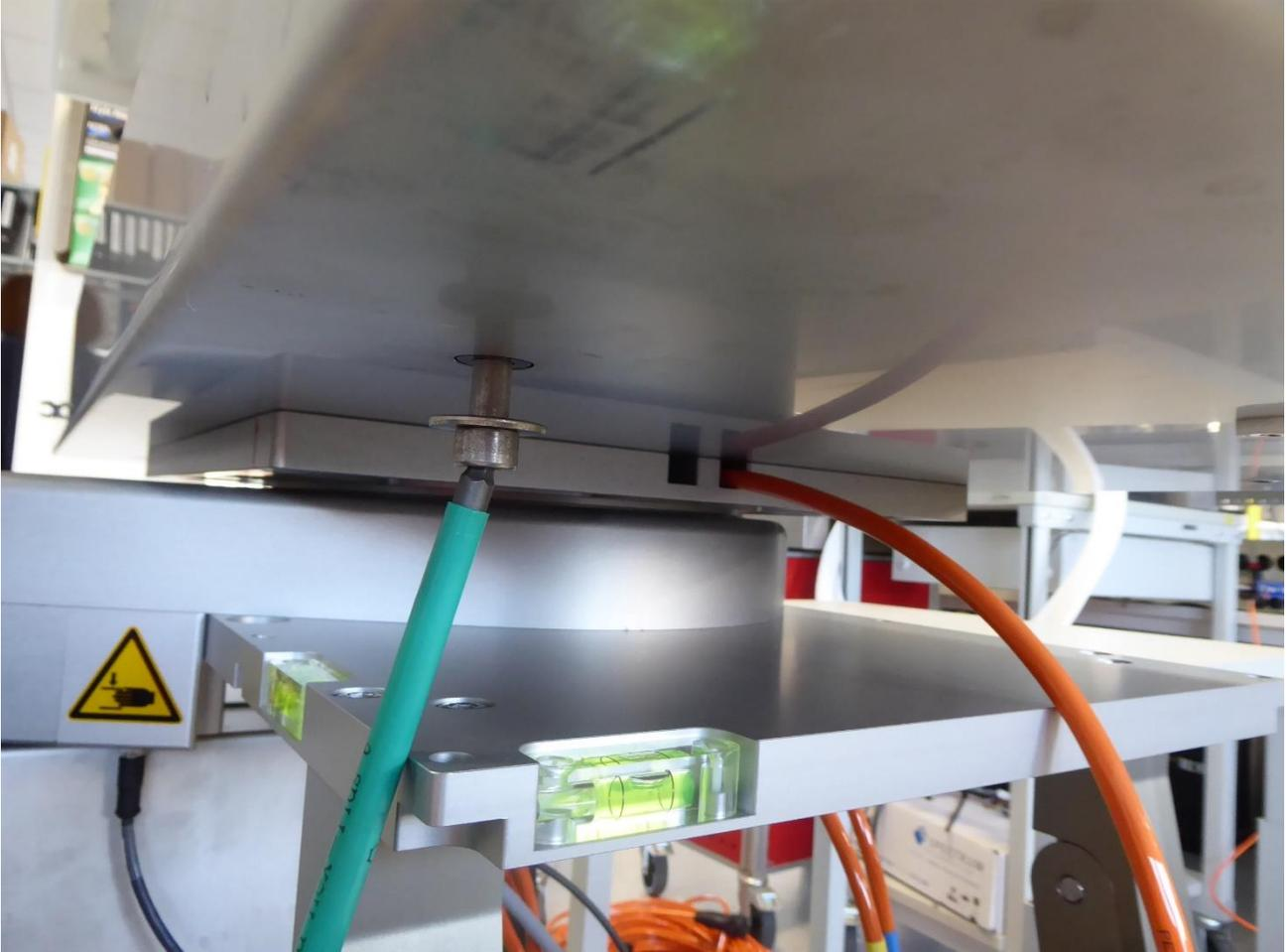
**Fig.2.5.15: mounting the 60mm screws using the 4 holes on the low temperature frame**
