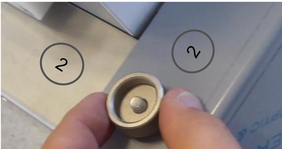
**(Fig.2.5.45): attach the knurled nuts to tight the frame**
