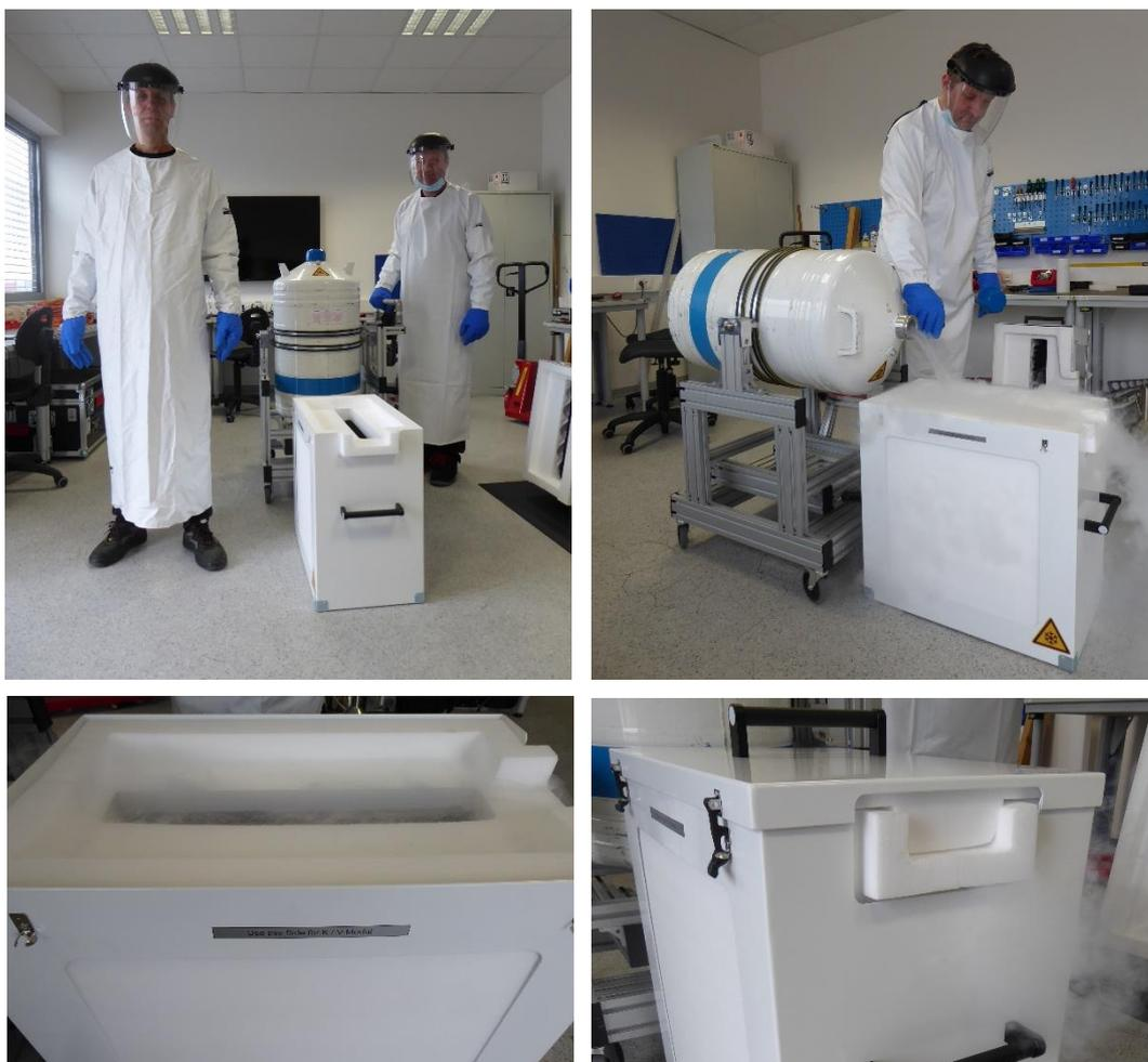
**Fig. 4.3.6: Fill the calibration target with LN<sub>2</sub> wearing suitable gloves, goggle and apron, check the filling level, close the lid, and fix the rubber fasteners.**
