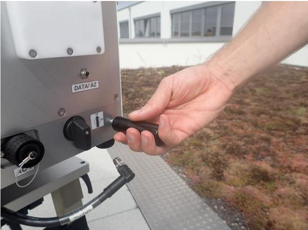
**Fig.2.5.15: remove the handles**
