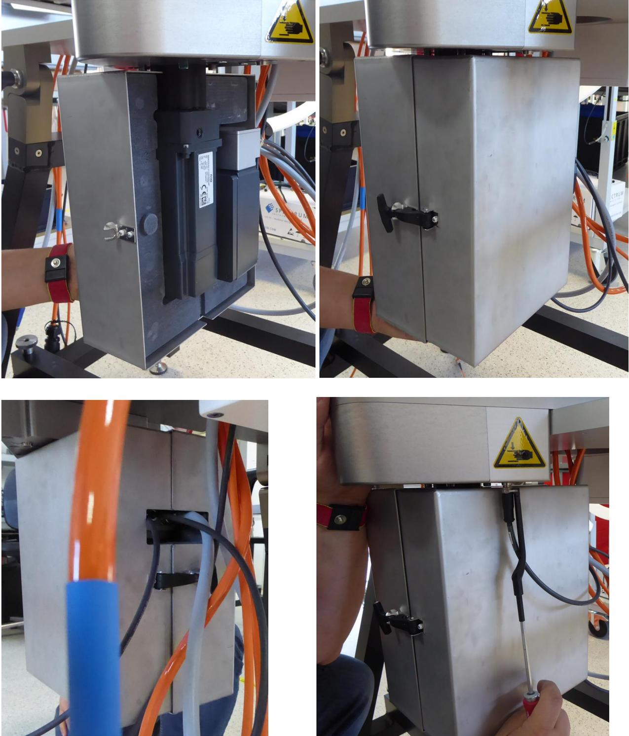
**Fig.2.4.10: mounted Azimuth insulation and fixing Azimuth drive cable**
