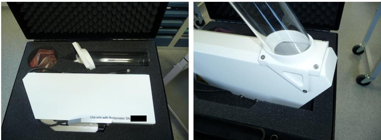
**Fig.2.6.9: IR Radiometer suitcase. Fix the protective glass tube gently to the housing, using 5 torx screws M4 x 20 mm.**
