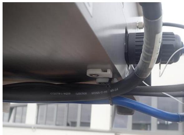
**Fig.2.5.18: Fastening cables on the radiometer's bottom plate.**
