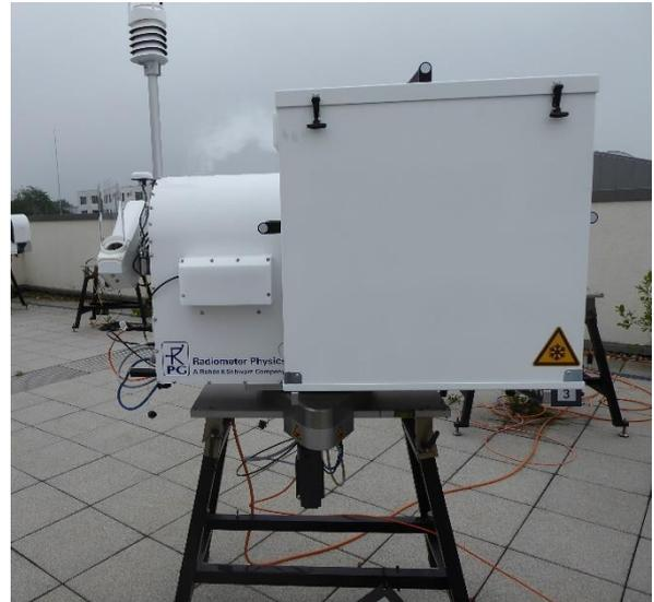
**Fig. 4.3.7: Place the target on the table. Make sure that the target's sidewall marked with "R1" is facing the radiometer.**
