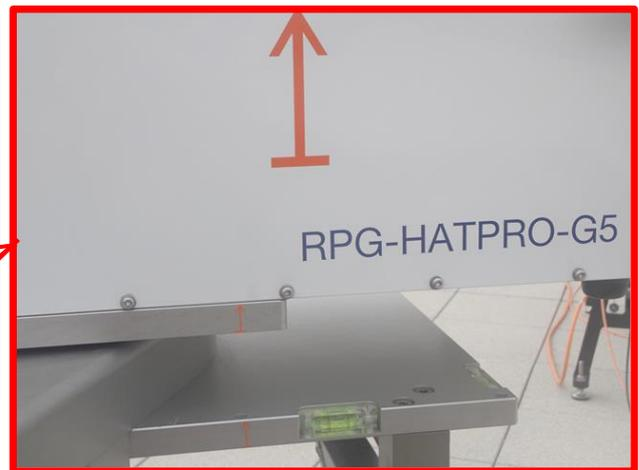
**Fig.2.5.13: mounting the radiometer on the low temperature frame**
