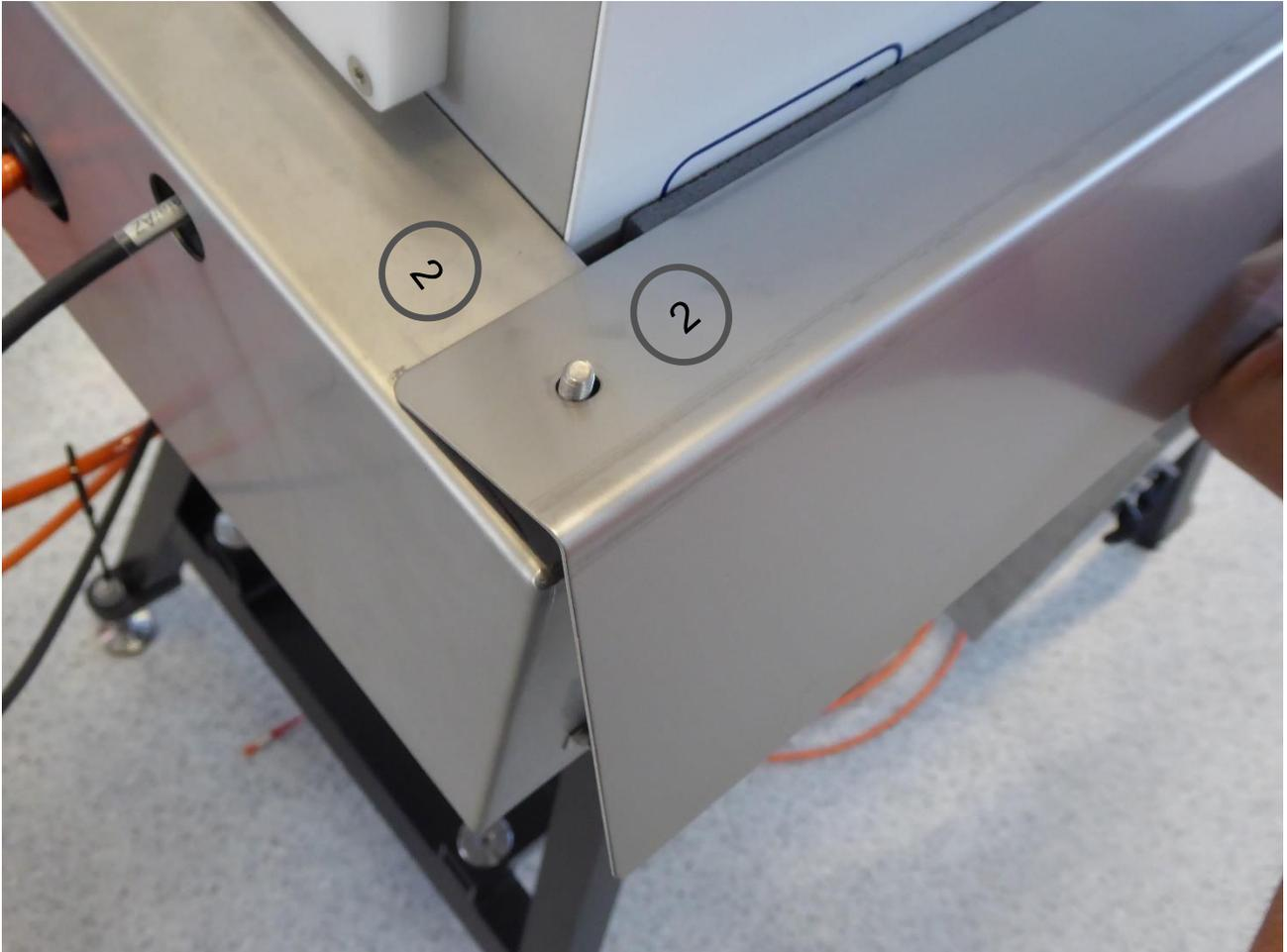
**(Fig.2.5.43): installation of the long frame unit marked with No. 2 and 3**
