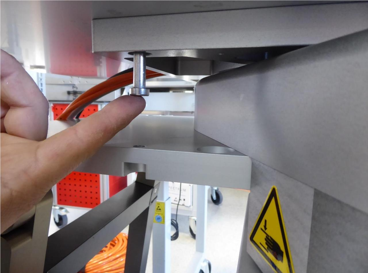
**Fig.2.5.14: mounting the 70mm screws using the 4 holes on the Azimuth drive**
