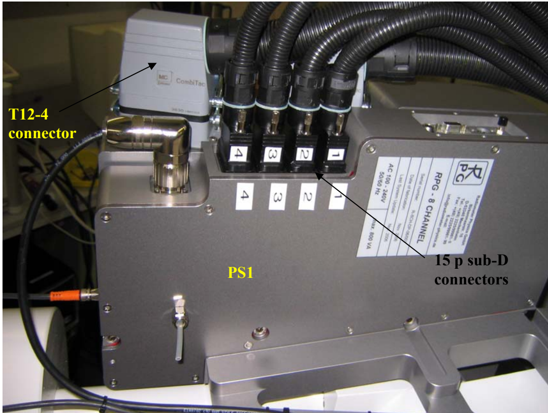
Fig.1.5: Connecting the receiver modules to PS1 / PS2.
