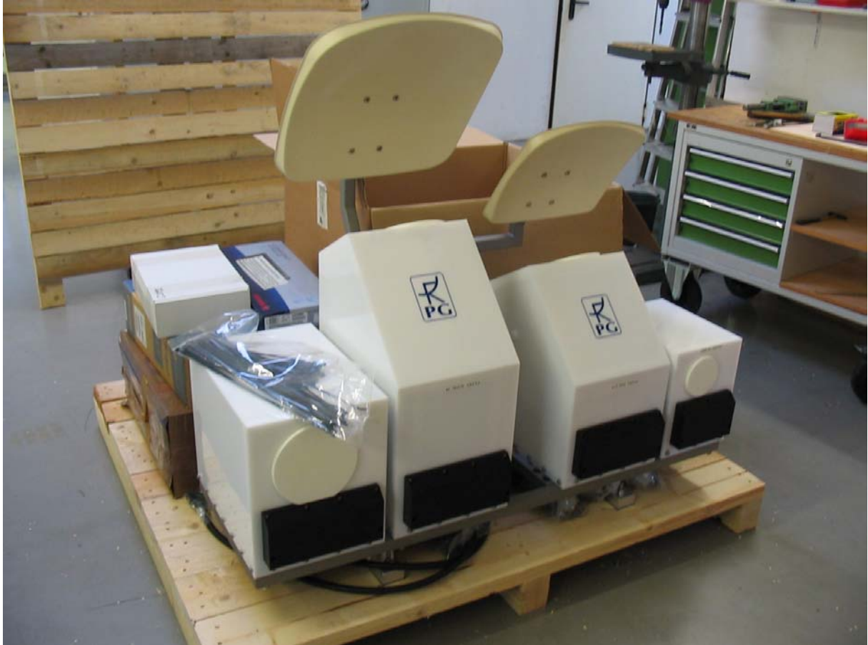
Fig.1.1: Content of box B. Radiometer modules are mounted to a steel frame that is also holding the two off axis parabola antennas for the low frequency channels.
