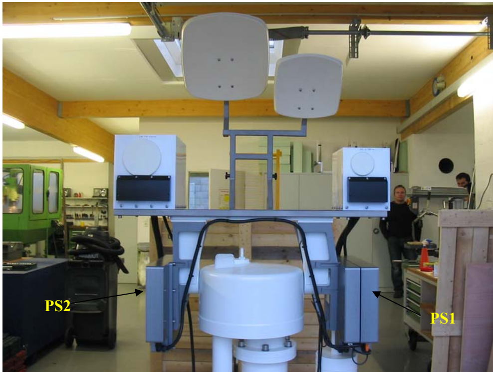
Fig.1.4: Mounting the main frame on top of the positioner's base plate.
