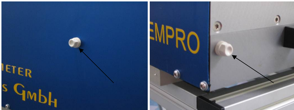
Fig.4.3.10: After the target frame has been unscrewed the open threads should be protected by plastic caps.
