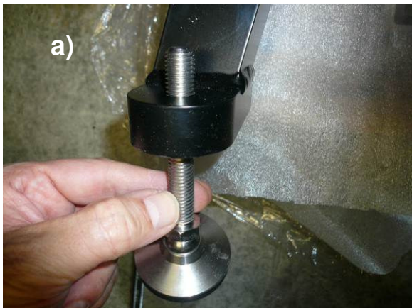
Fig.2.3.2: Mounting the feet to the stand's legs.
