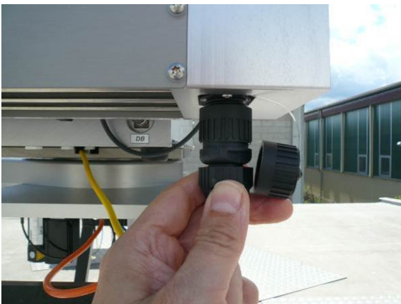
Fig.2.6.7: Connection of AC2 cable (yellow) to the heater module AC input.
