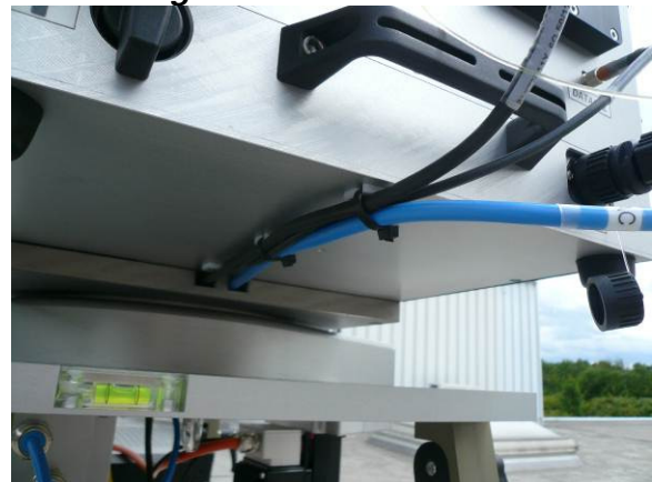
Fig.2.5.10: Fastening cables on the radiometer's bottom plate.
