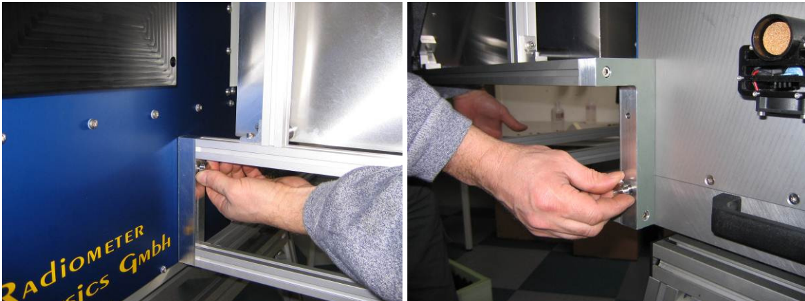
Fig.4.3.5: location of mounting screws for the target frame.
