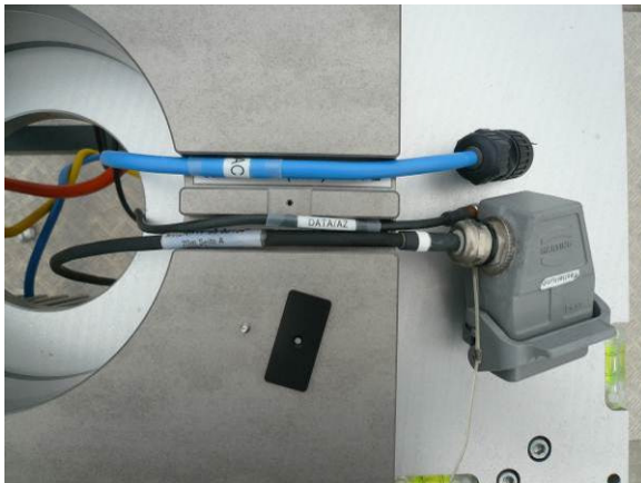
Fig.2.4.11: Mounting the cables into the cable channels.
