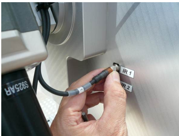
Fig.2.6.10: Connecting the IRRs to their interface ports (IR1 and IR2).
