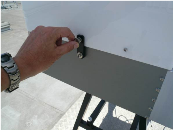
Fig.2.6.5: Shift the heater module underneath the blower's air inlet and fasten the mounting screws as indicated.
