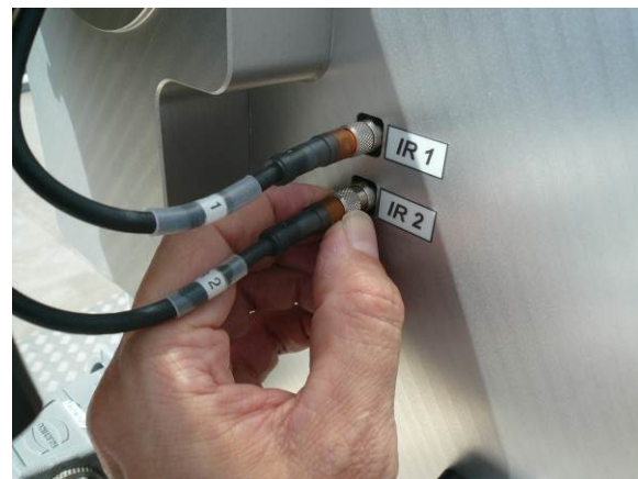
Fig.2.6.10: Connecting the IRRs to their interface ports (IR1 and IR2).
