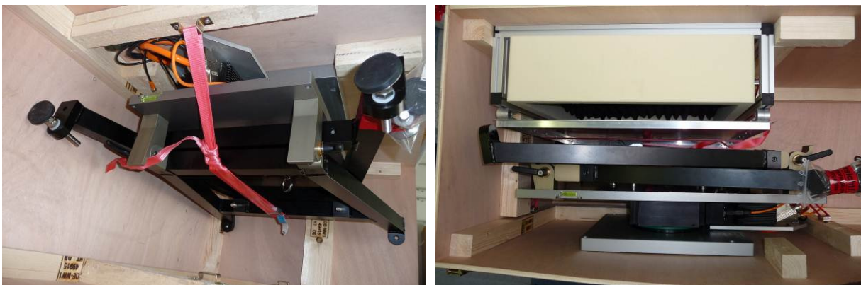
Fig.2.2.3: Folded stand fastened to the side wall and packing of calibration target
