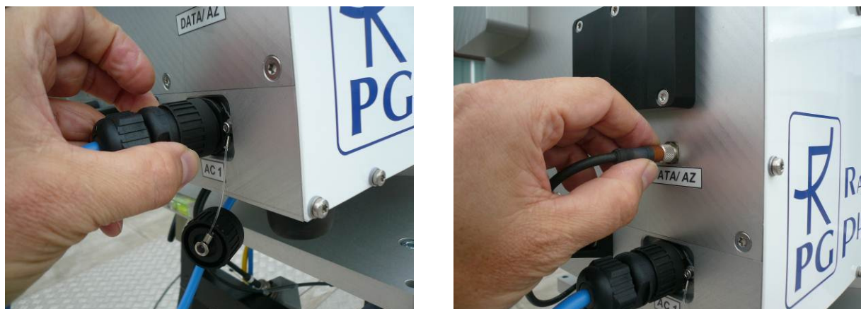
Fig.2.5.6: Connecting the blue AC1 cable and the black azimuth driver interface cable (DATA/AZ).
