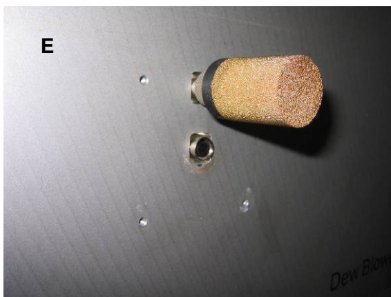
Fig.4.4.1: Dismounting the external surface sensors: A) Sensor cage below the dew blower. B) Unscrewing the T-sensor fan. C) Unscrewing the sensor cage housing. D) The humidity sensor (with gold plated cap) and the temp. sensor can be unscrewed by hand. E) Temperature sensor removed. F) Humidity sensor removed.
