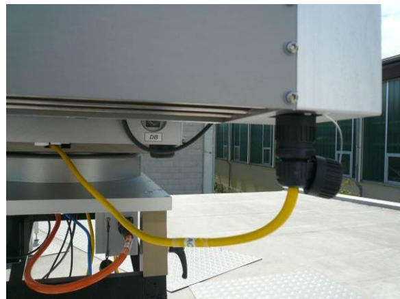
Fig.2.6.7: Connection of AC2 cable (yellow) to the heater module AC input.
