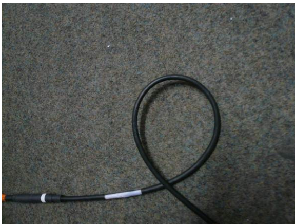
Fig.2.8.2: Avoid loops in the fibre optics cable. The curvature radius should not be less than 5 cm. Crossings of cables can lead to cable damage when stepping on it.
