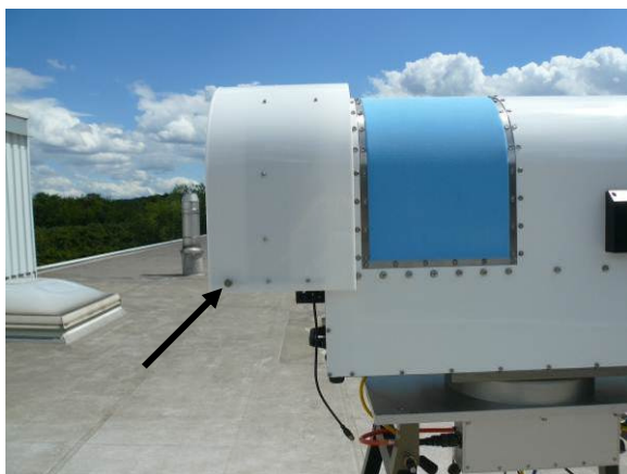
Fig.2.6.4: Remove heater mounting screws from the blower.
