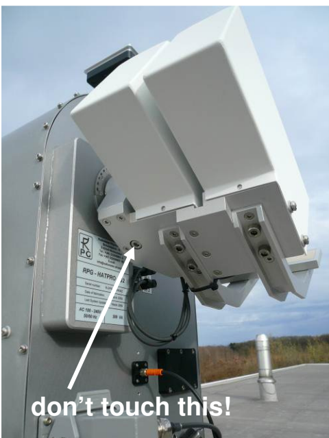
Fig.2.6.12 For the motorized IR-Option (Option IRR-B), the IR radiometers are mounted with three M4 screws (A). NEVER touch the screw in (B). It has been adjusted to an elevation axis tilt accuracy of 0.3°. By loosening (B), this adjustment is lost.
