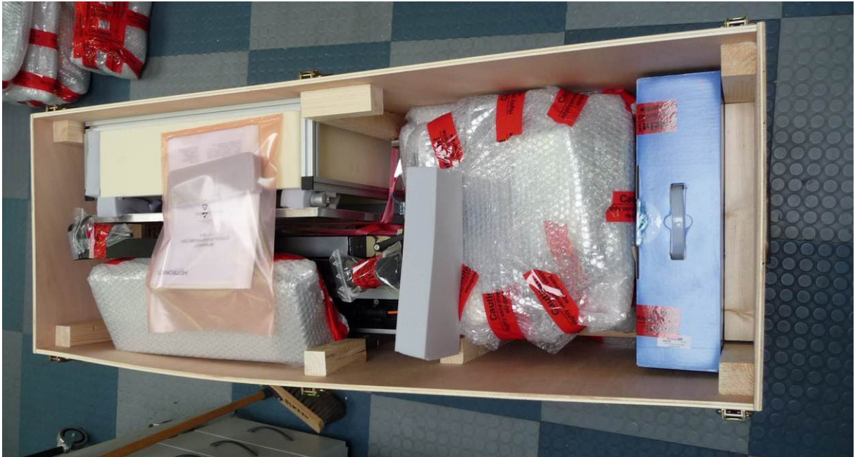
Fig.2.2.2: Accessory box with radiometer stand, calibration target, heater module, cables, IR Radiometer, azimuth drive and host PC (including monitor, keyboard).
