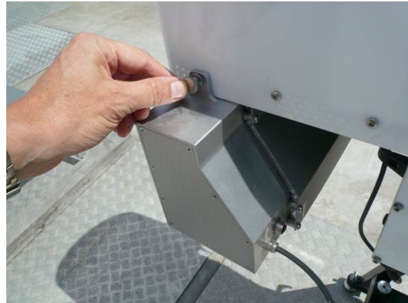
Fig.2.6.5: Shift the heater module underneath the blower's air inlet and fasten the mounting screws as indicated.
