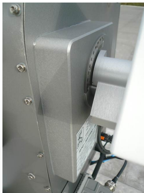
Fig.2.6.12 For the motorized IR-Option (Option IRR-B), the IR radiometers are mounted with three M4 screws (A). NEVER touch the screw in (B). It has been adjusted to an elevation axis tilt accuracy of 0.3°. By loosening (B), this adjustment is lost.
