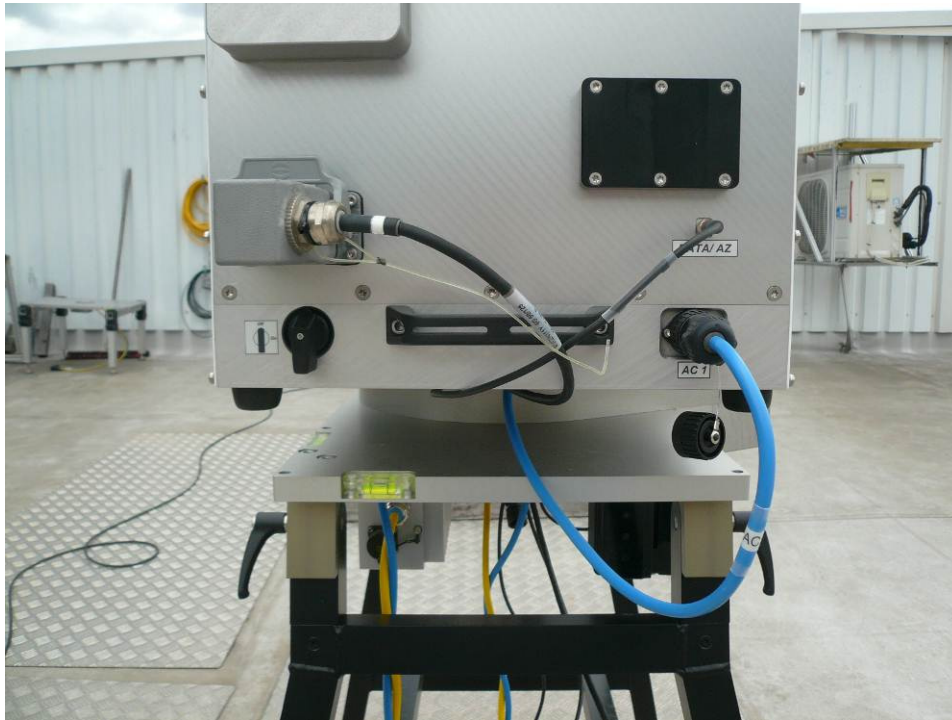
Fig.2.5.8: All cables connected to the radiometer.
