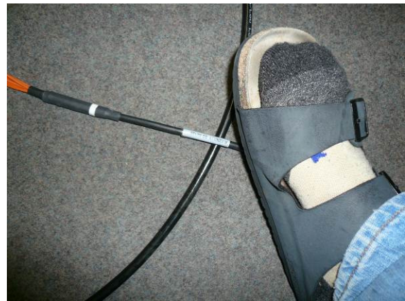
Fig.2.8.2: Avoid loops in the fibre optics cable. The curvature radius should not be less than 5 cm. Crossings of cables can lead to cable damage when stepping on it.
