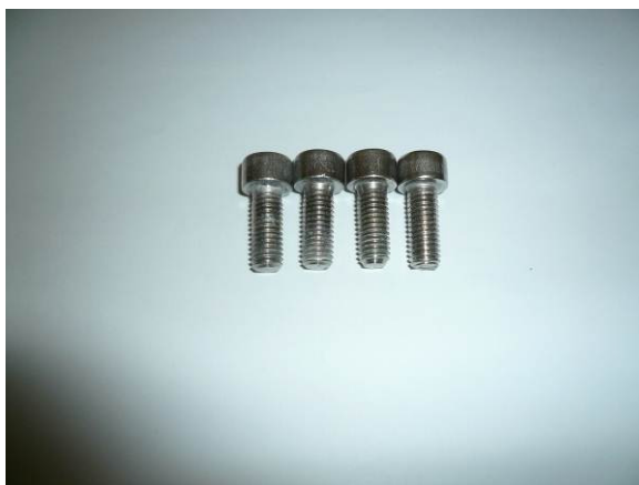
Fig.2.5.2: Four M8x20 screws for fixing the radiometer box on the azimuth driver table.
