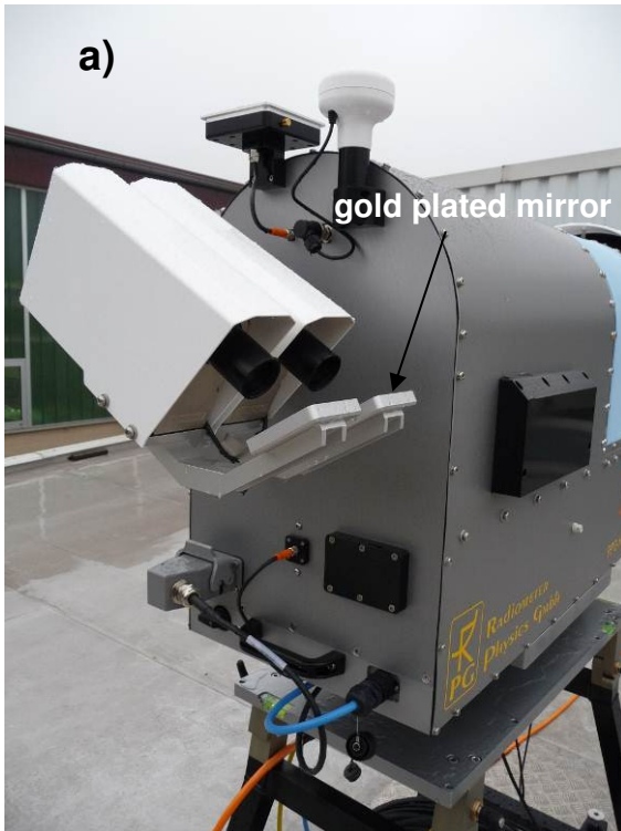
Fig.2.6.9: Infrared radiometer mounted to the radiometer side wall on manually adjustable elevation axis. Because of an axial mount the IR radiometer viewing angle can be changed between 0° and 90° and fixed at an arbitrary angle in this range.
