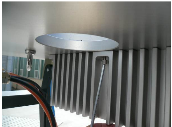
Fig.2.4.4: 6 M6x20 screws for mounting the azimuth drive power supply (on the right).
