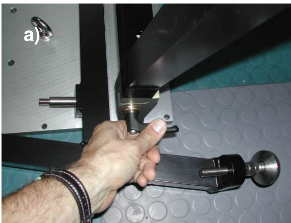
Fig.2.3.4: Open clamps and turning legs into upright position.
