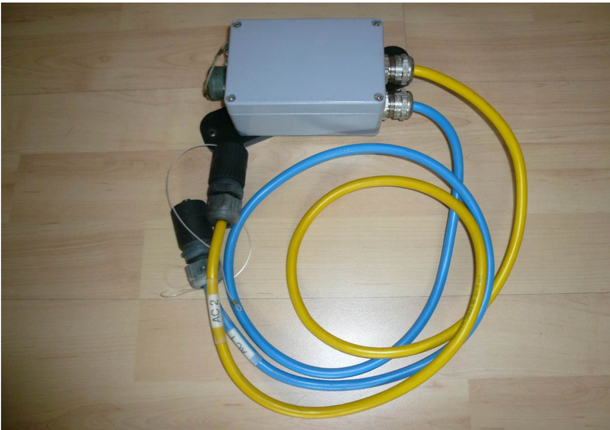
Fig.2.4.7: Power splitter unit used instead of the power supply in Fig.2.4.4, if no azimuth positioner option is installed.
