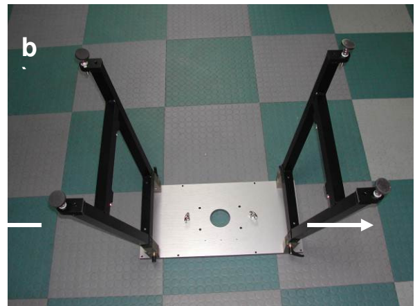
Fig.2.3.4: Open clamps and turning legs into upright position.
