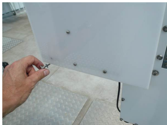
Fig.2.6.4: Remove heater mounting screws from the blower.
