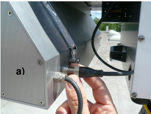
Fig.2.6.6: Connect blower supply to heater module (a) and then connect heater module to radiometer ( b), 'DB' connector socket).
