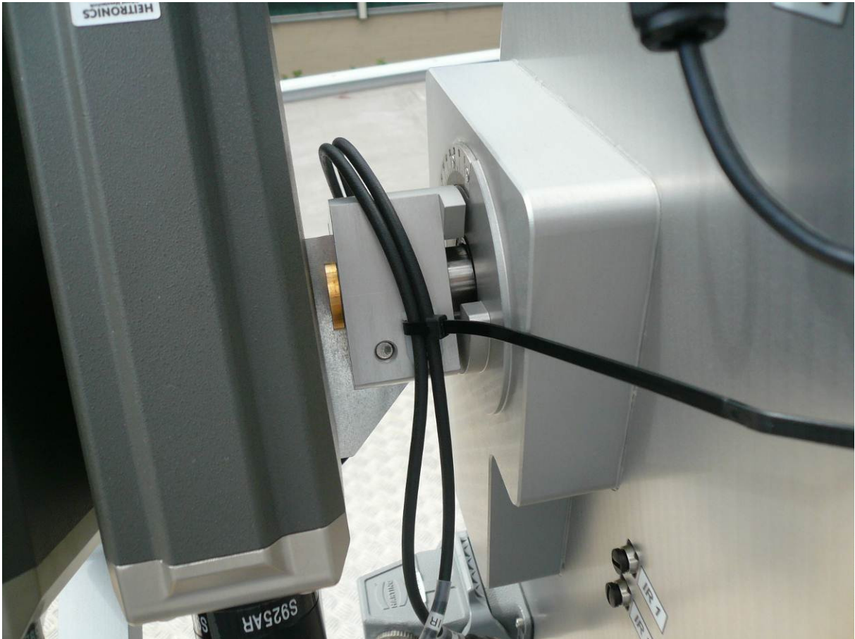
Fig.2.6.13: Also fasten the IR-interface cables with a cable tie.
