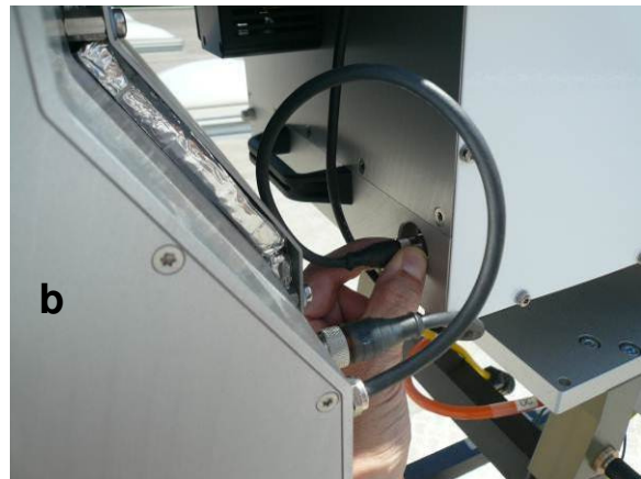
Fig.2.6.6: Connect blower supply to heater module (a) and then connect heater module to radiometer ( b), 'DB' connector socket).
