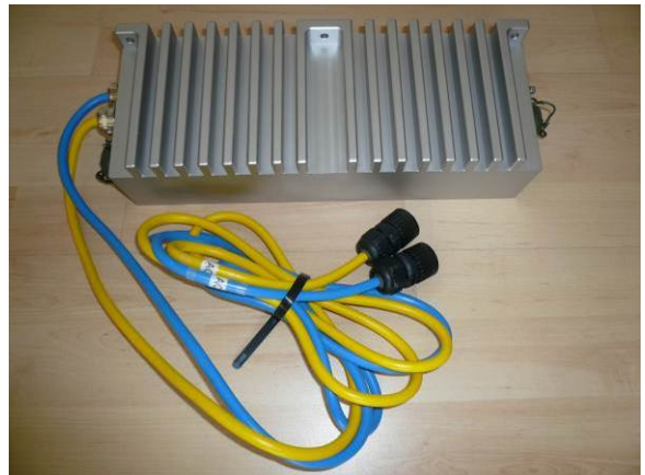
Fig.2.4.4: 6 M6x20 screws for mounting the azimuth drive power supply (on the right).
