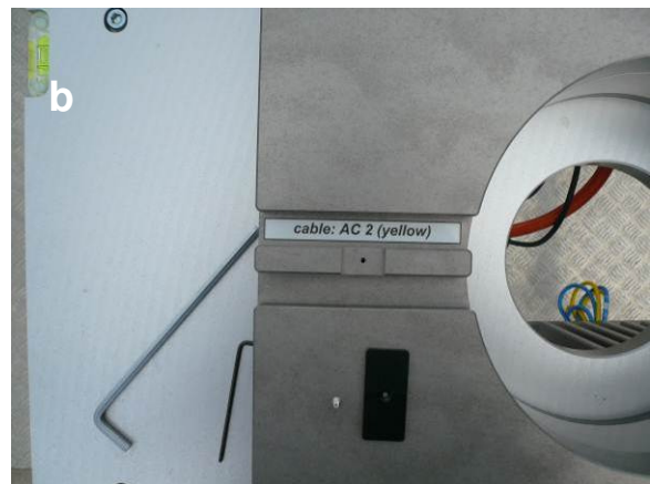
Fig.2.4.9: Labeled cable channels for a): AC1 cable (blue), DATA/AZ cable (black), fiber optics DATA cable (black) and b): AC2 cable (yellow).
