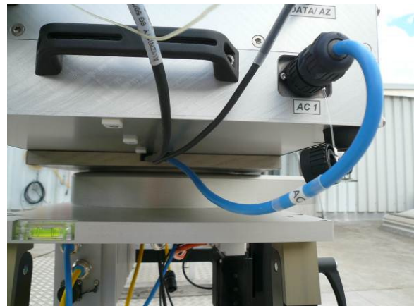
Fig.2.5.9: Pulling back the cables to adjust the cable lengths.
