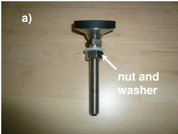
Fig.2.3.1: One of the four stand's feet.
