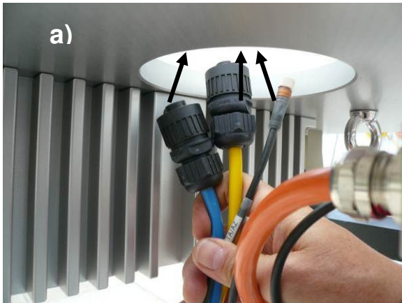
Fig.2.4.10: Feeding AC1, AC2, DATA/AZ and fibre optics data cable through centre hole.
