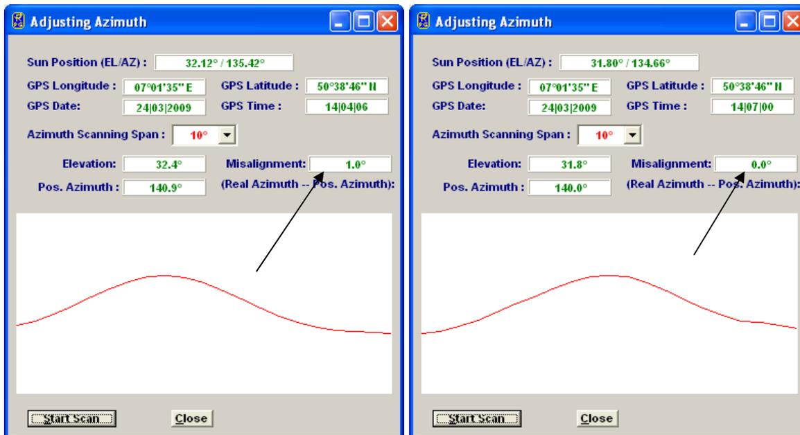
**Fig.4.33: Azimuth angle adjustment using the sun position.**
