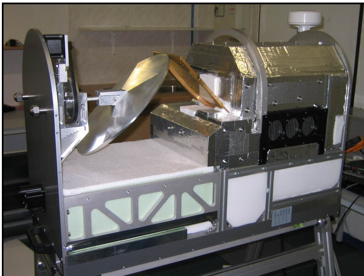
Fig.2.6: Extensive insulation of all receiver components in combination with a two-stage stabilisation system allows to achieve a thermal receiver stability of 30 mK over the full operating temperature range.
