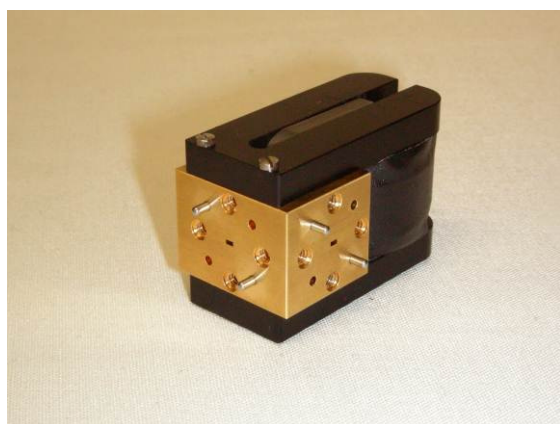
Fig.2.2f: Left: Narrow band 90 GHz y-junction Dicke Switch (transmission loss 0.6 dB, right: Full W-band Faraday Dicke Switch (transmission loss 1.0 dB).
