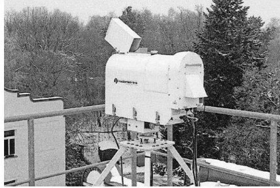
FIG. 1. The microwave profiler TP/WVP-3001.
