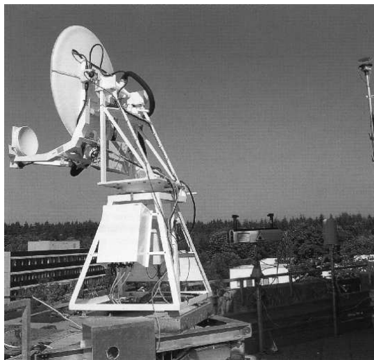
Figure 5.1: The 19 GHz radiometer on top of the roof: The antenna is aligned to southward direction with an elevation of 30 degree. On the right hand side the meteorological sensors can be seen.
