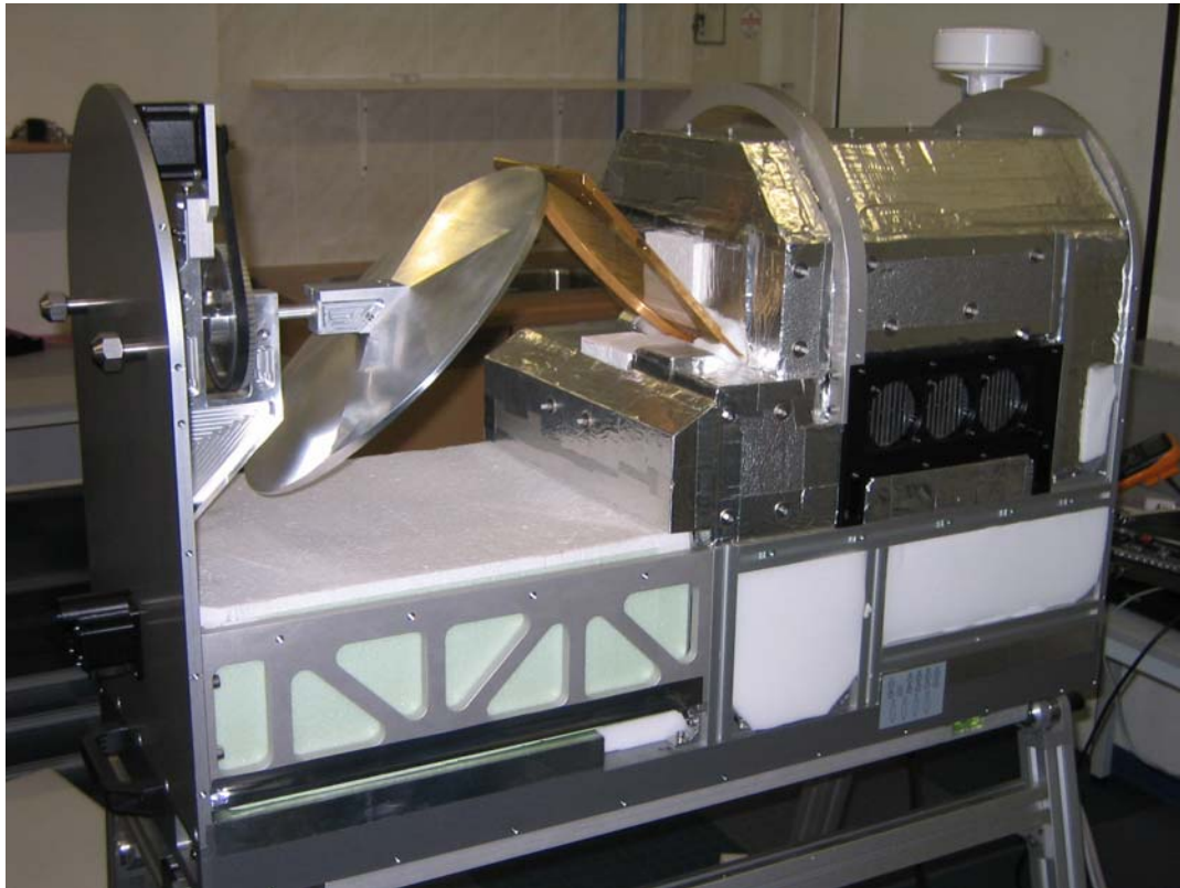
Thermal insulation plus two stage thermal control system stabilizes the receiver temperatures to better than 30 mK.
