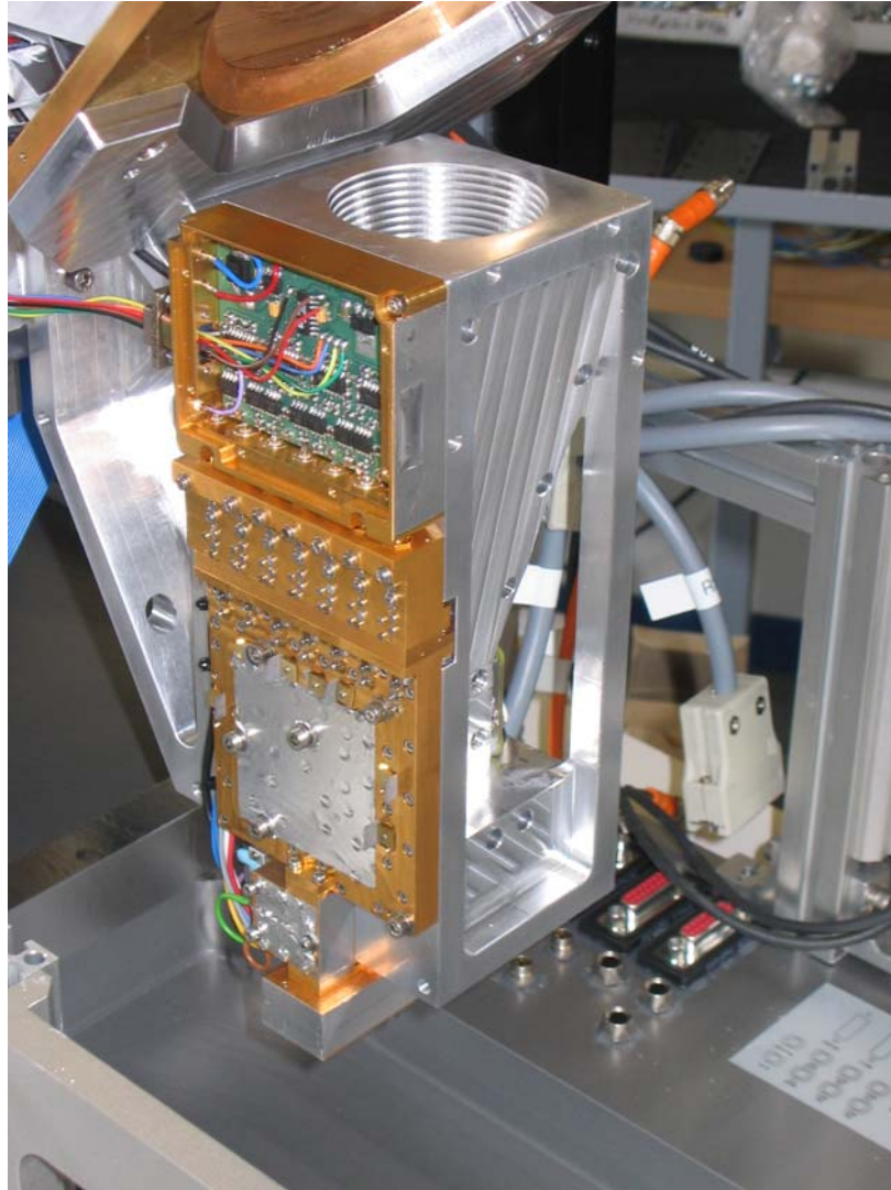
Compact V-band DDFB receiver including feedhorn, noise injection, Dicke switch, LNAs, 7-way power splitter, detector section, video amplifiers and 16 bit ADC section. The system is realised all in waveguide technology to avoid SMA connectors that would reduce the system stability.
