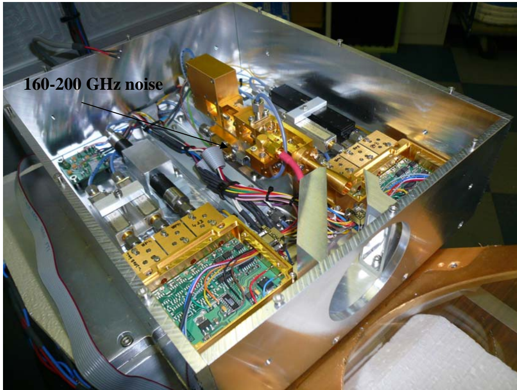
6 channel 183 GHz water vapour radiometer including noise source for auto-calibration.
