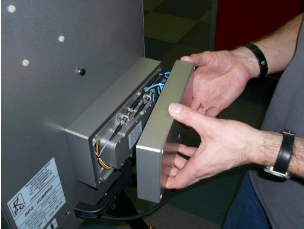
Fig.8.15a: Mounting of the lid.
