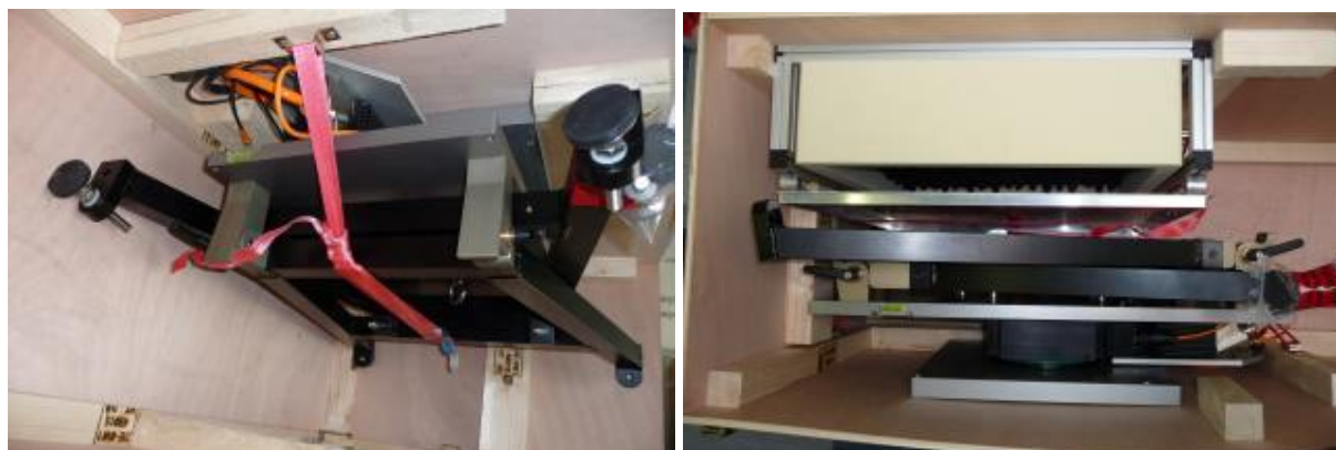
Fig.1.3: Folded stand fastened to the side wall and packing of calibration target
