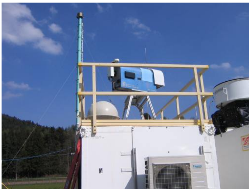
Figure 34: A HATPRO instrument with azimuth positioner during full sky scan operation at the US ARM mobile facility.
