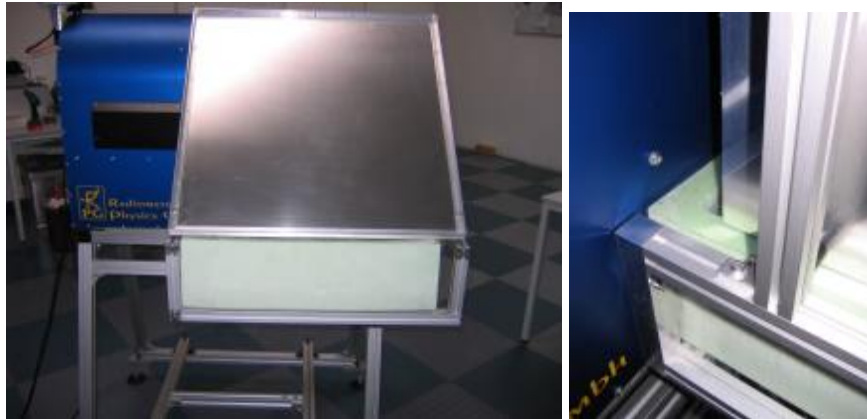
Fig.4.5d: Push the target to its final position.
