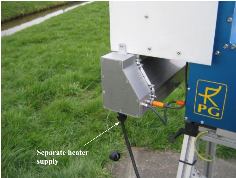
Fig.8.2: Dew blower heater module mounted to the blower air inlet using three of the blower's housing screws. Also shown are the electric connections.
