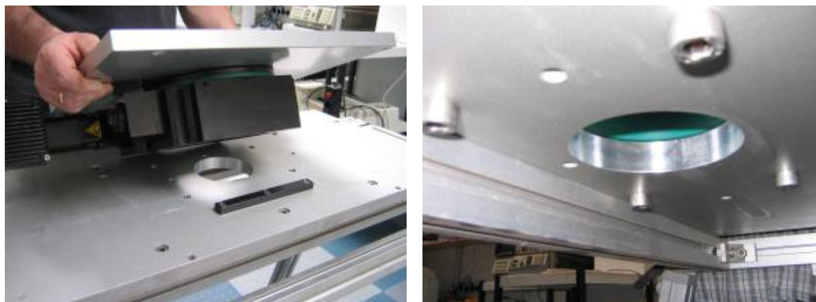
Fig.8.5: Mounting the positioner and adapter plate on the modified stand.
