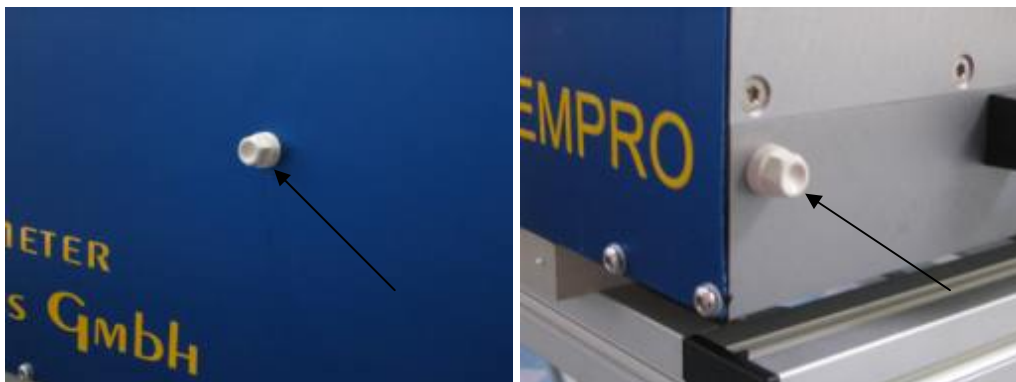
Fig.4.6: After the target frame has been unscrewed the open threads should be protected by plastic caps.
