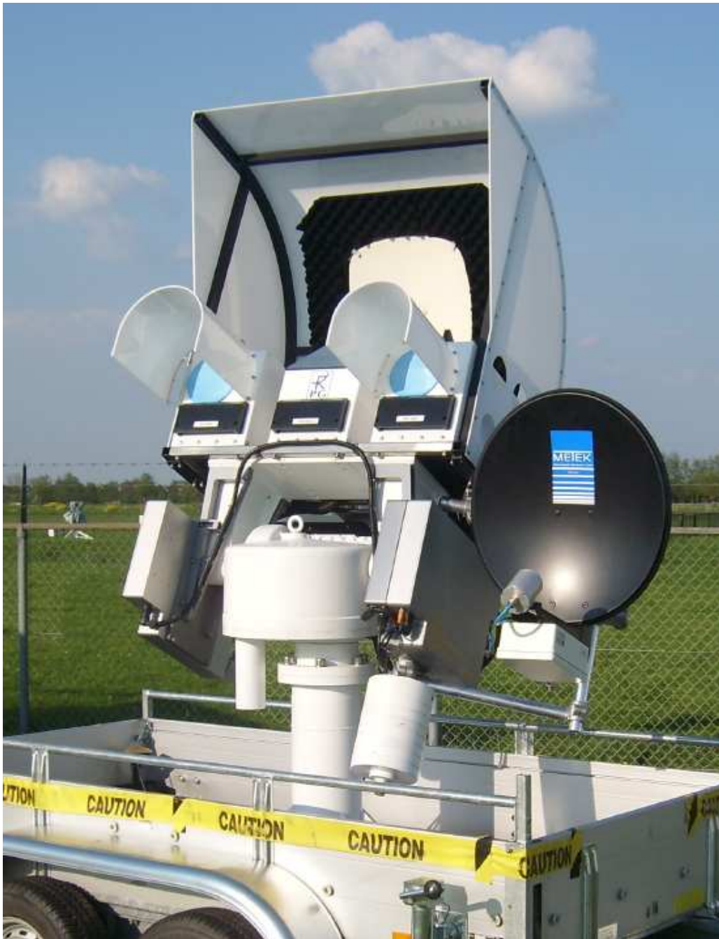
FIG. 1. The ADMIRARI radiometer at the CESAR observatory. On the right side (black antenna) a Micro Rain Radar system is installed.
