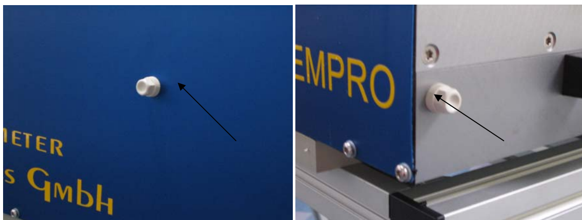
Fig.4.6: After the target frame has been unscrewed the open threads should be protected by plastic caps.
