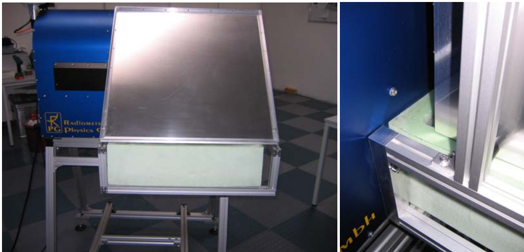
Fig.4.5d: Push the target to its final position.
