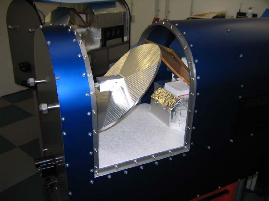
Fig.7.6: Radiometer with removed microwave window.
