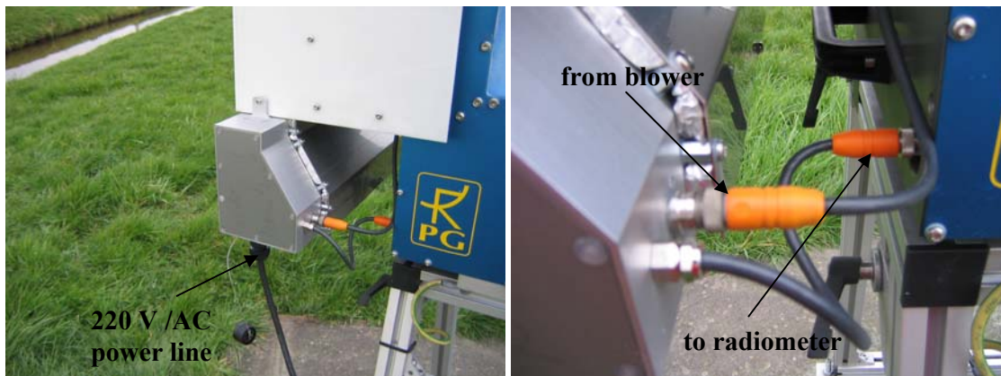
Heater mounted to the blower unit. The blower supply cord is connected to the heater instead of the radiometer and the heater is directly plugged into the radiometer box. The heater is powered via an AC power cable and consumes 2 kW of power. Voltage: 220 V/AC (for US or Japanese customers we provide a transformer 110 V → 220 V).
