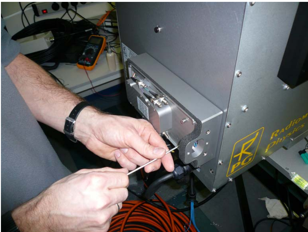
Fig.8.12b: Screw converter A to radiometer housing using the 50 mm screws contained in the upgrade kit.
