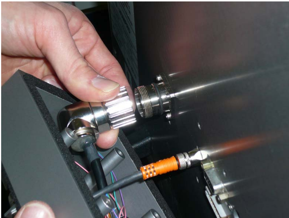
Fig.8.11: Connect converter A to radiometer.
