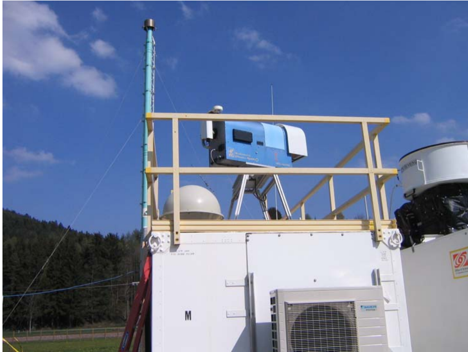
Figure 34: A HATPRO instrument with azimuth positioner during full sky scan operation at the US ARM mobile facility.
