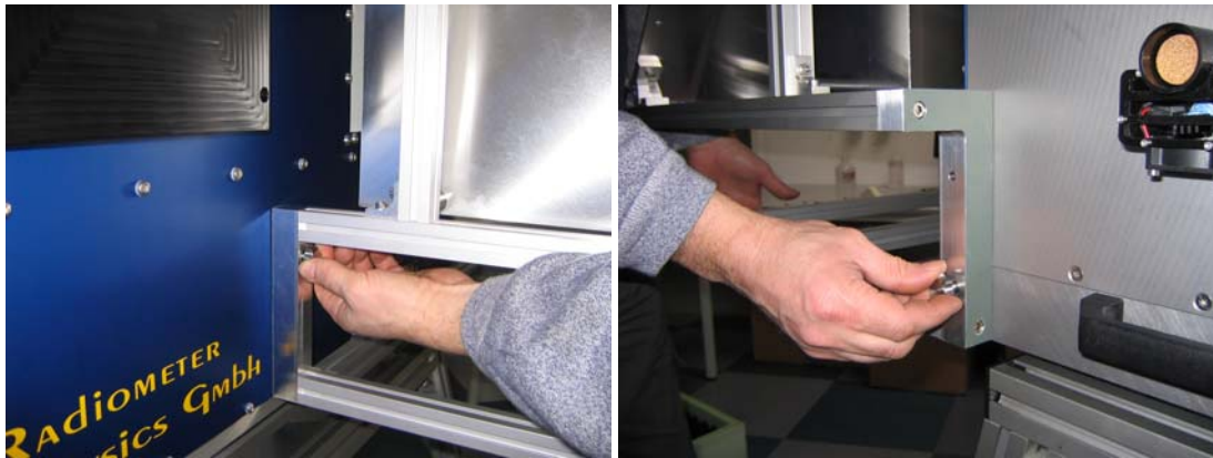
Fig.4.5a: location of mounting screws for the target frame.
