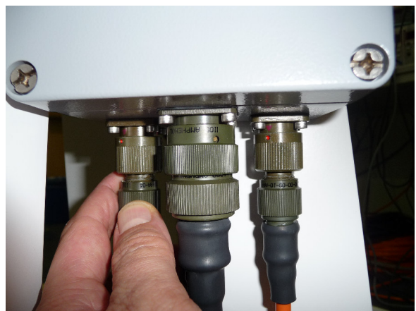
Fig.1.1.1f: On the left side, unplug the following connectors from the El / Az controller unit: X2, X3, X4, X5, AC IN. Then unscrew the unit.
