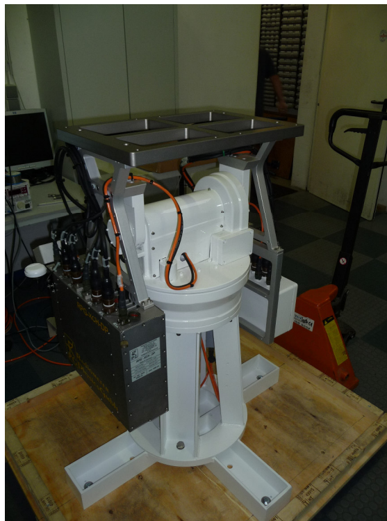
Fig.1.1.1c: Unscrew the frequency modules from the top mounting frame.
