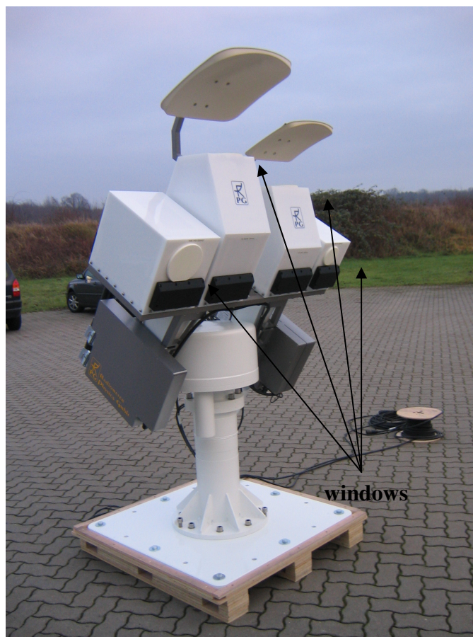
Fig.6.1: Location of the microwave windows for cleaning.
