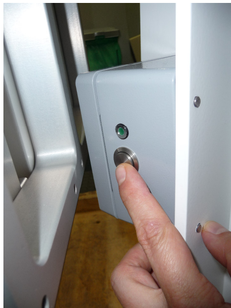
Fig.1.1.1a: Turn off the radiometer power first (if radiometer is turned on).
