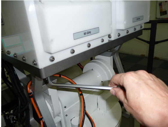
Fig.1.1.1c: Unscrew the frequency modules from the top mounting frame.
