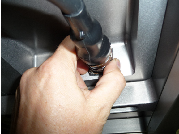
Fig.1.1.1b: Unplug the frequency modules' data and power cables.
