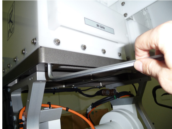
Fig.1.1.1c: Unscrew the frequency modules from the top mounting frame.
