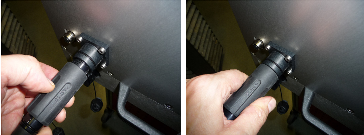
Fig.1.2.1c: Plug in 2 line fibre optics connector.
