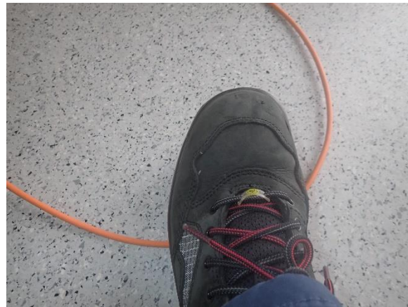
Fig.2.8.2: Avoid loops in the fiber optics cable. The curvature radius should not be less than 5 cm. Crossings of cables can lead to cable damage when stepping on it.
