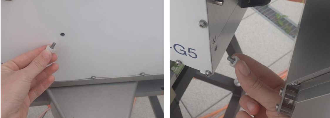
Fig4.3.10: After calibration and dismantling of the calibration target, make sure that the protection screws are inserted again.
