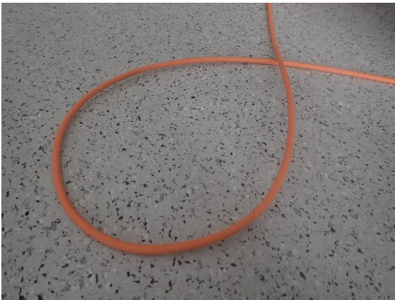
Fig.2.8.2: Avoid loops in the fiber optics cable. The curvature radius should not be less than 5 cm. Crossings of cables can lead to cable damage when stepping on it.
