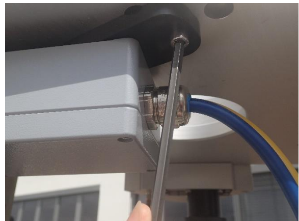
Fig. 2.4.4.: Fixing the power splitter unit to the bottom side of the stand with 2 M6x20 screws.
