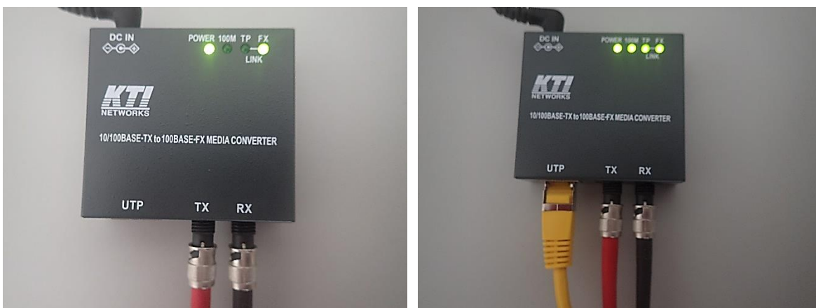
Fig.2.7.3: 2 line fiber optics to LAN-TCP/IP converter.
