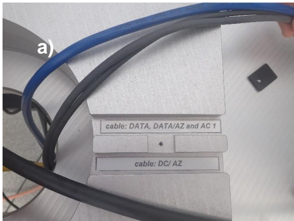
Fig.2.4.6: Labeled cable channels for a): AC1 cable (blue), DATA/AZ cable (black), fiber optics DATA cable (black) and DC/AZ cable and b): AC2 cable (yellow).
