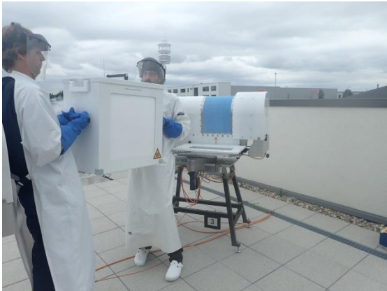
Fig.4.3.5: Turn the radiometer by 180° so that “R2” side of the target is facing the radiometer now.
