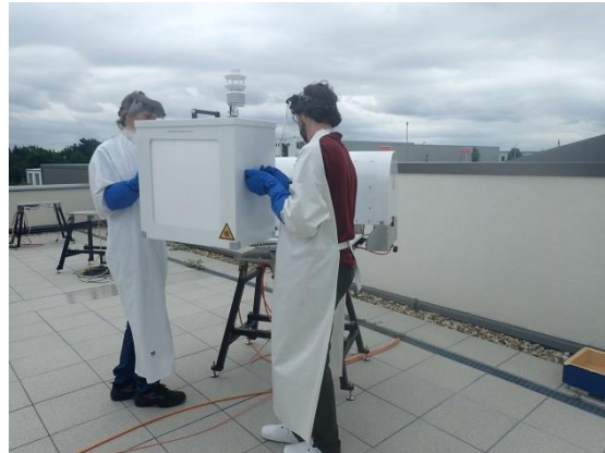
Fig.4.3.5: Turn the radiometer by 180° so that “R2” side of the target is facing the radiometer now.
