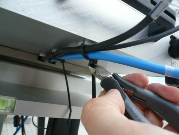
Fig.2.5.10: Fastening cables on the radiometer's bottom plate.
