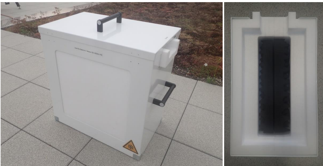
Fig. 4.3.2: Cold calibration target PT-V1 container (left) and blackbody absorber (right).
