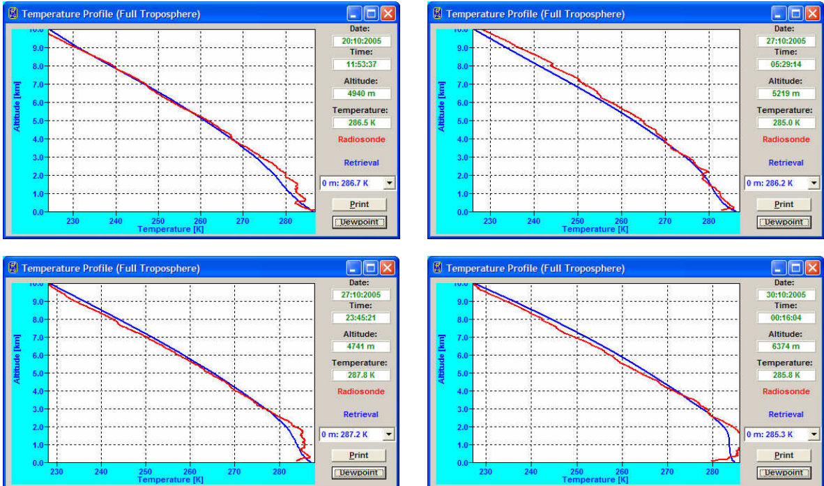
Fig.2.14a: Examples of comparisons between radio sounding (red) and HATPRO Z mode observations (blue). The boundary layer details are not always accurately resolved.
