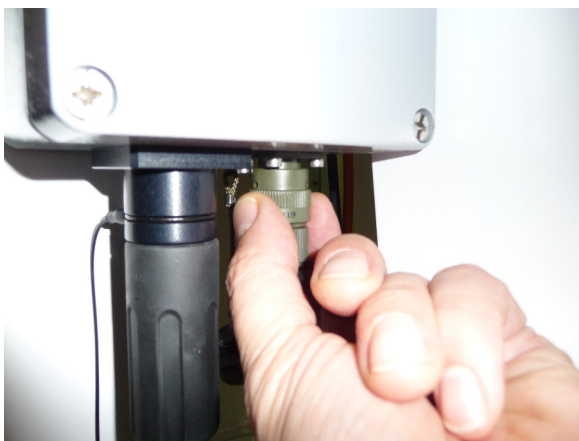
Fig.1.1.1f: On the left side, unplug the following connectors from the EI / Az controller unit: X2, X3, X4, X5, AC IN. Then unscrew the unit.
