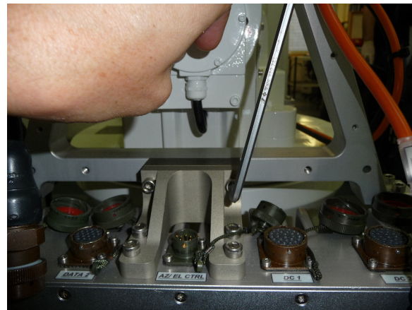
Fig.1.1.1e: Unscrew the main control unit from the holding frame.
