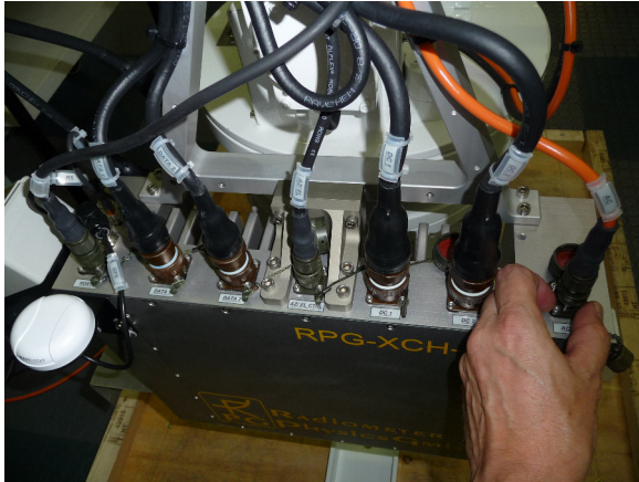
Fig.1.1.1d: On the right side, unplug the following connectors from the main control unit: HOST, DATA1, DATA2, AZ / EL CTRL, DC1, DC2, AC.
