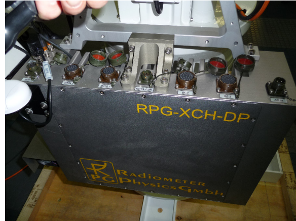
Fig.1.1.1d: On the right side, unplug the following connectors from the main control unit: HOST, DATA1, DATA2, AZ / EL CTRL, DC1, DC2, AC.
