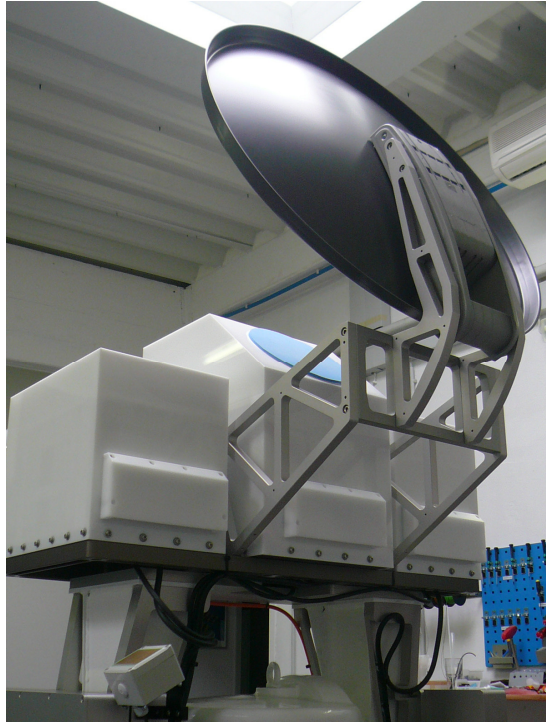
Fig.1.1b: Parabola antenna mount structure used for 6.925 / 10.7 GHz combination modules.
