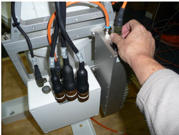
Fig.1.1.1f: On the left side, unplug the following connectors from the EI / Az controller unit: X2, X3, X4, X5, AC IN. Then unscrew the unit.
