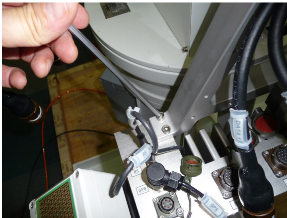
Fig.1.1.1e: Unscrew the main control unit from the holding frame.
