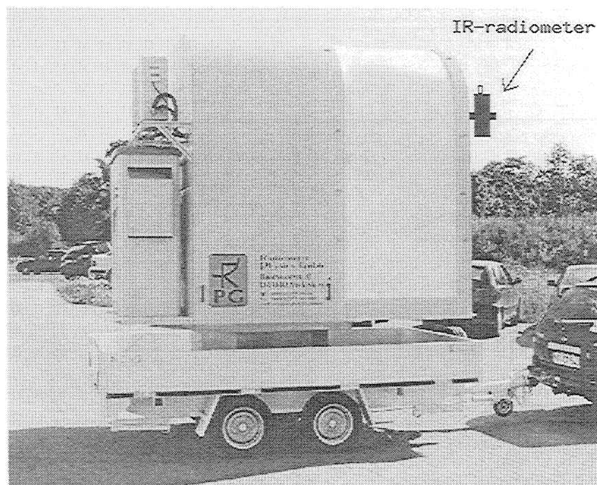
Figure 3. Photograph of the transportable microwave radiometer MICCY. The position of the infrared radiometer mounted on the antenna axis is indicated.
