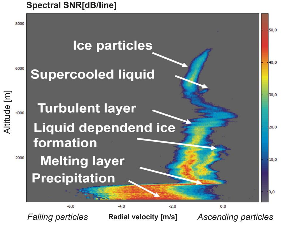
In the single polarization configuration the melting layer is used for a basic classification of scatter types. The dual polarization configurations allow for more reliable detection of the melting layer and detailed particle categorization.
