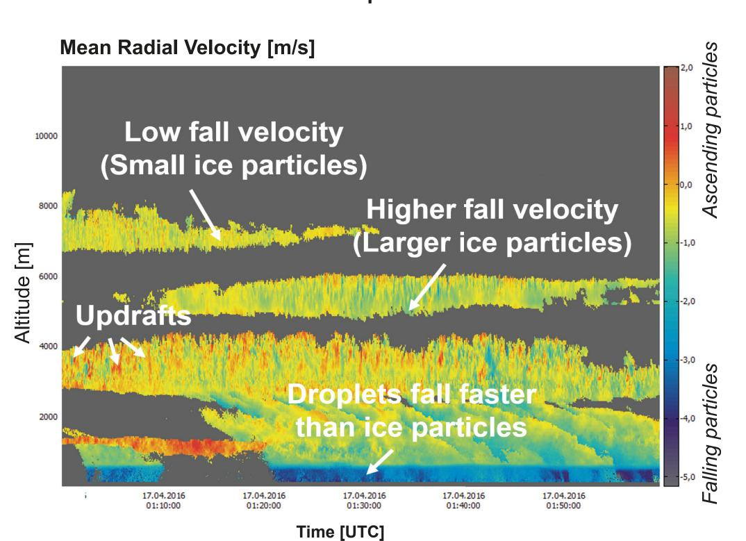
Turbulent areas of the atmosphere are dangerous for regional airlines. As the radar has Doppler capabilities, it allows for a detection of turbulence and wind shears. Therefore, the cloud radar is a valuable source of additional warning information for civil aviation.
