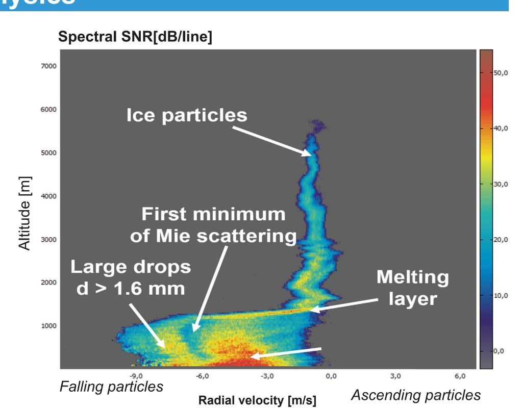
In the case when the size of liquid drops exceed 1 mm, resonance scattering effects occur. This provides a reference for size determination of raindrops even in light intensity precipitation.
